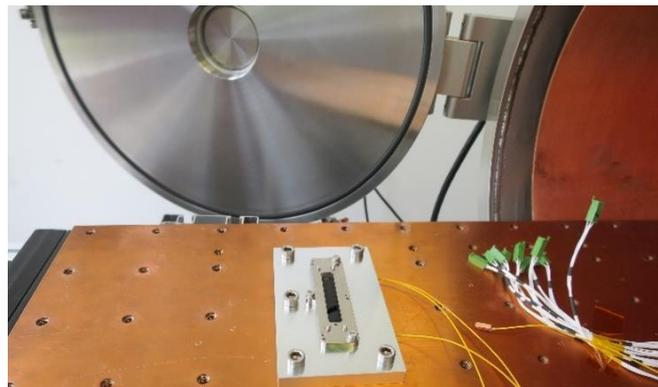
Figure 16: SLIDS on thermal adapter of thermal vacuum chamber
