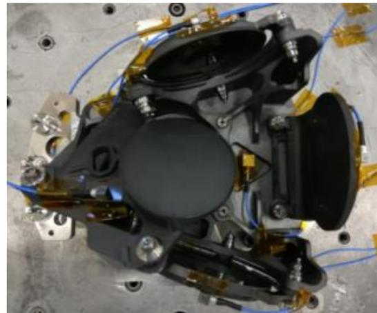
*Scanner (engineering model) and derotator (mechanical model)*
