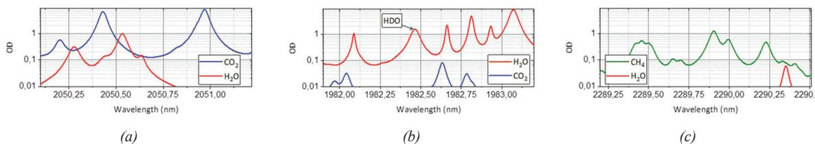
Figure 3. Optical depth calculated within the three main spectral windows of interest with HITRAN 2016 for a 6 km two-way vertical path (from ground). CO<sub>2</sub> window (a), water vapor and HDO window (b), CH<sub>4</sub> window (c).
