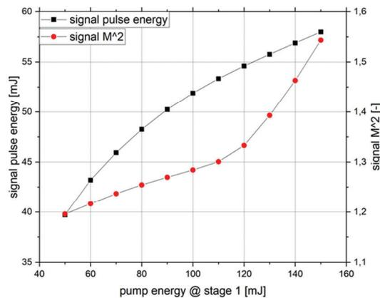
Figure 6. Extracted signal beam energy and  $M^2$  calculated at the output of the OPA line as a function of pump energy in the first OPA stage. The configuration is composed of two stages with two PPKTP crystals in each stage and idler filtering. The total pump energy distributed in the OPA line (stage 1+2) is 200 mJ.
