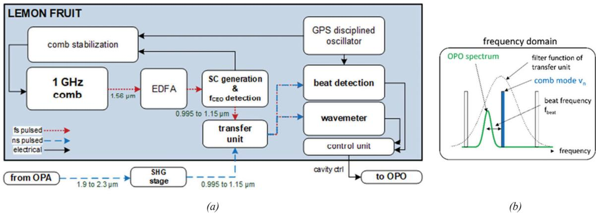
Figure 8. LEMON Frequency Reference Unit (FRUIT) principle diagram (a). Beat note measurement principle (b). EDFA is Erbium Doped Fiber Amplifier, SC stands for Super Continuum, and SHG for Second Harmonic Generation.
