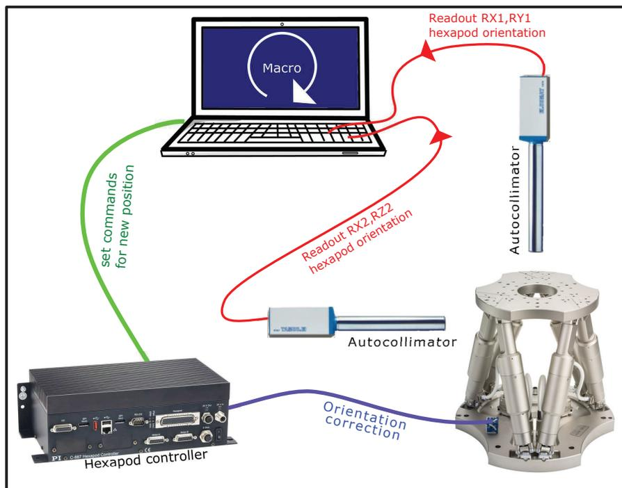
Figure 6. Orientation feedback loop principle realized at XPBF 2.0 and re-used by MINERVA.
