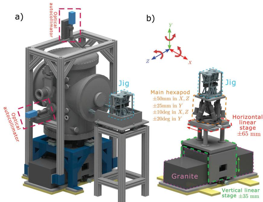
Figure 5. Sample environment. In a) is shown the vacuum chamber surrounded by a aluminum structure supporting the 2 autocollimators. In b) mechanical solution to limit the number of hexapod orientation corrections.
