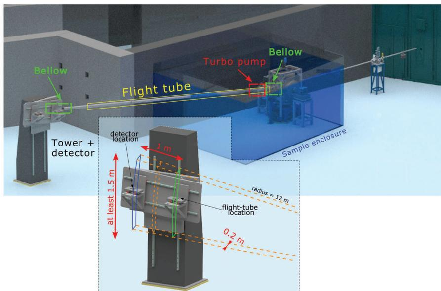
Figure 7. Flight tube connecting the vacuum chamber inside the sample enclosure and the detector tower. The detector positioning mechanism allows all the suitable degrees of freedom to intercept the deflected beam by any kind of MM necessary for the ATHENA optics.
