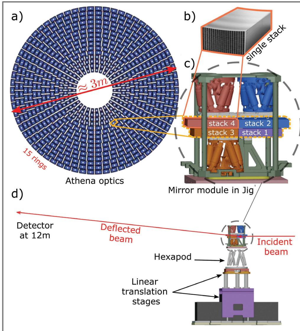
Figure 1. The ATHENA optics made of 15 rings and populated by about 700 mirror modules a). Stack produced by cosine with the Silicon Pore Optics technology b). Mechanical Jig with 4 stacks to be aligned with a collimated X-ray beam c). Principle of measurement of a whole MM at MINERVA d).
