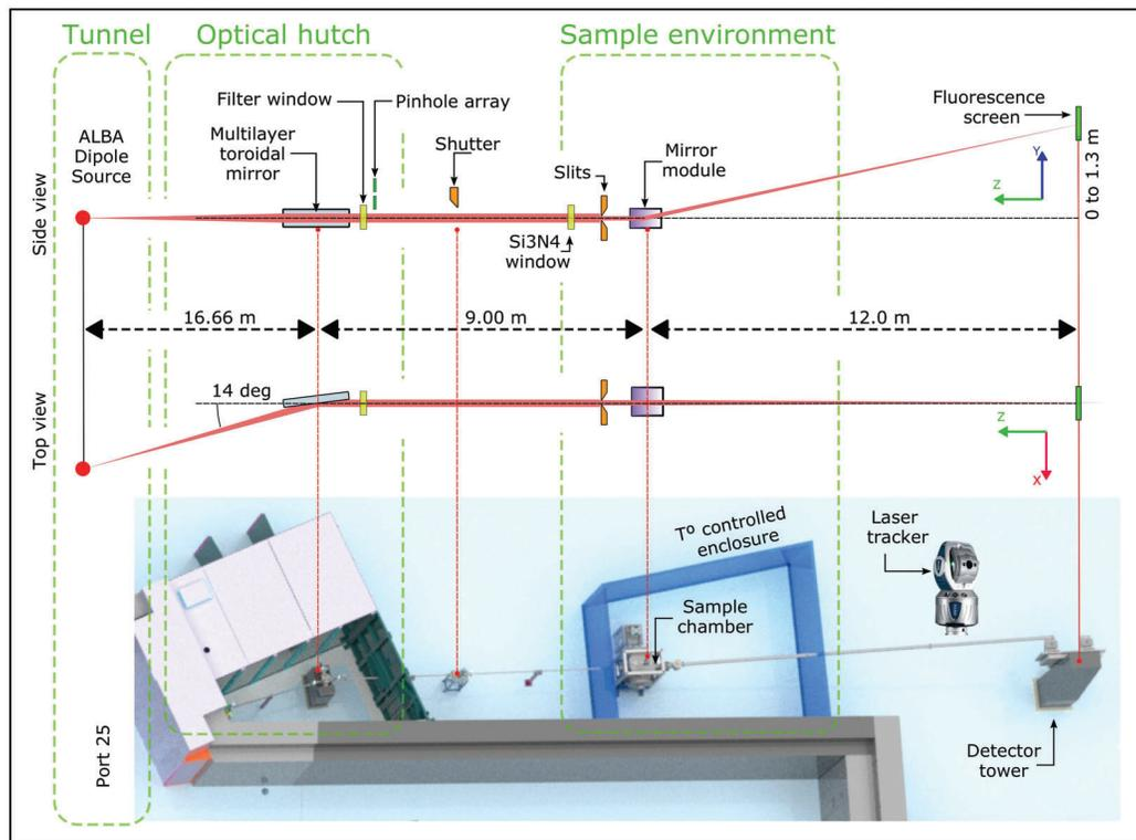
Figure 2. MINERVA layout presenting the main components of the beamline. Side view in a), top view in b) and 3D view in c).
