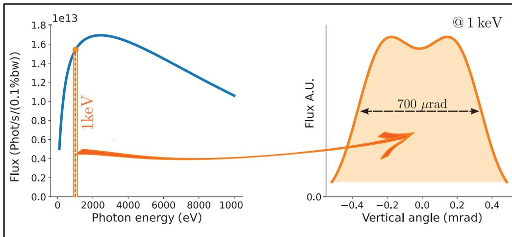
Figure 3. a) Spectral flux delivered by the ALBA bending magnet with 1 mrad horizontal acceptance and 250 mA electron beam current. The flux at 1 keV is approximately  $1.5\text{e}13$  photons/sec/0.1%bw. b) The vertical angular distribution is about  $700 \mu\text{rad}$  at 1 keV. Calculations performed by XOPPY.<sup>12</sup>
