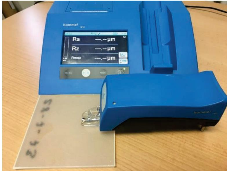
Figure 12. Profilometer Hommel Etamic W10 used for the SR measurements.
