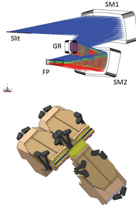
Figure 7. Top: Each CHIME SU Optical design comprises two freeform mirrors (SM1, and SM2) and a broadband, spherical, diffraction grating (GR). Bottom: The staggered arrangement of the three SUs defining the SE.
