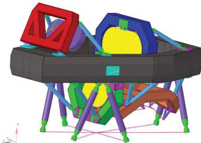
Figure 9. Structural architecture showing the central optical bench torus (black) to which the other units attach
