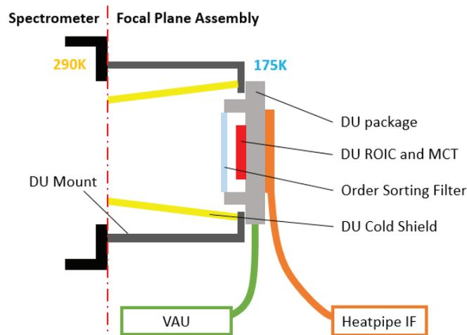
Figure 11. Detector Focal Plane Assembly
