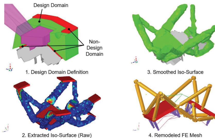
Figure 10. Topology Optimization Process flow from the design space definition to the remodeled FE model
