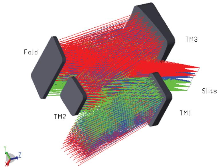
Figure 4. The telescope optics: a TMA of Wetheral-Womble type with powered mirrors TM1, TM2 and TM3, and a fold mirror at which focus correction can be applied during flight.
