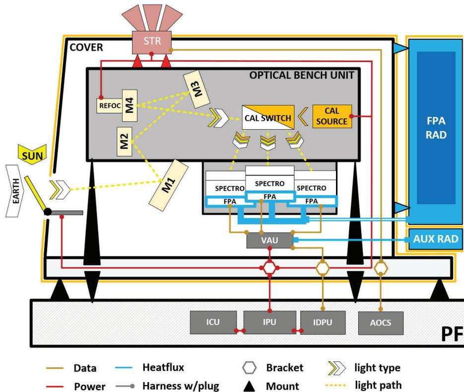
Figure 2. Instrument layout diagram with the two light paths for earth observation (white arrows) and calibration (sun calibration yellow, spectral calibration orange).
