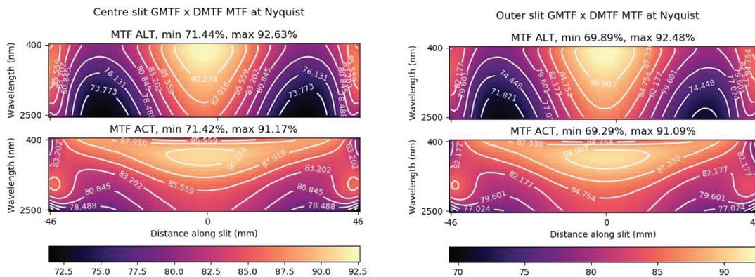
Figure 6. Tangential (ALT) and sagittal (ACT) MTF at the detector’s Nyquist frequency of 13.88 cycles per millimeter, over the full detector from 400 nm to 2500 nm for the combined telescope and spectrograph for (left) the centre spectrograph unit, and (right) the outer spectrograph (where performance is lowest) for the current optical design. The asymmetry introduced by the telescope is evident in the right-hand figure.
