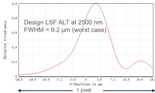
Figure 8. Line spread function of the spectrometer along track at 2500nm.
