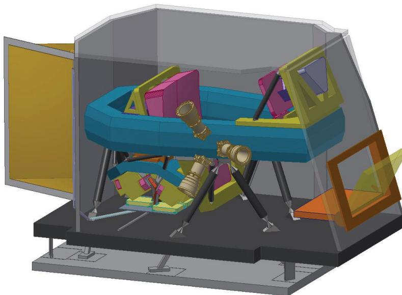
Figure 1. CHIME Instrument Architecture Concept Overview
