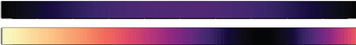
Figure 5. Wavefront error map: Center slit (top) with range 80.4 nm to 134 nm. Outer slits (lower) with WFE range 45 nm to 284 nm. In the outer slits, the WFE is highest at the innermost ends of the slits (light colour); in the centre slit the WFE is highest in the centre of the slit.
