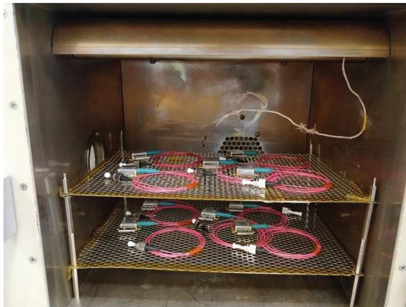
Figure 2-6 Thermal test chamber
