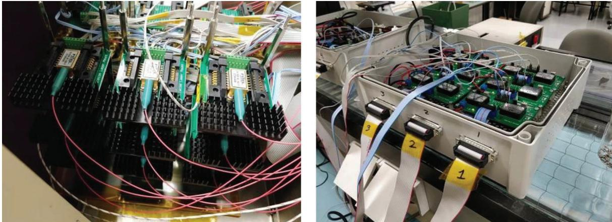
Figure 2-7 Endurance test setup. Left: Lasers mounted in sockets . Right: Thermo-electric controllers.
