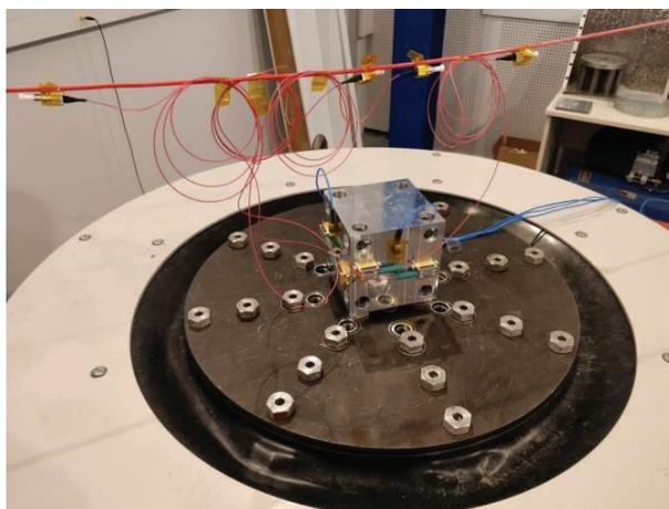
Figure 2-5 Vibration test setup
