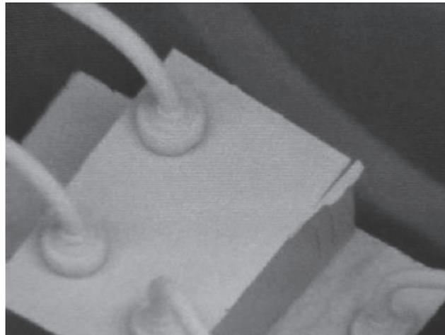
Figure 2-8 SEM picture of laser chip, showing small piece of top metallization remaining after die cutting.
