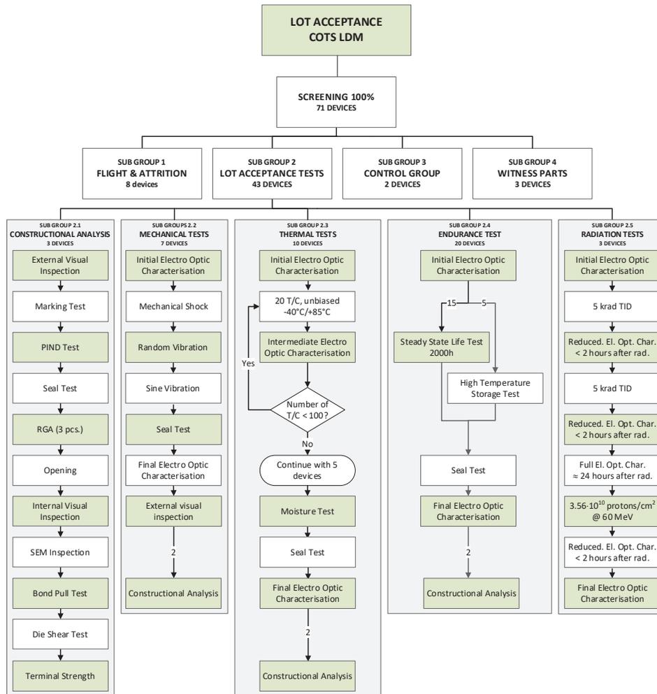
Figure 2-1 LDM LAT Test flow.
