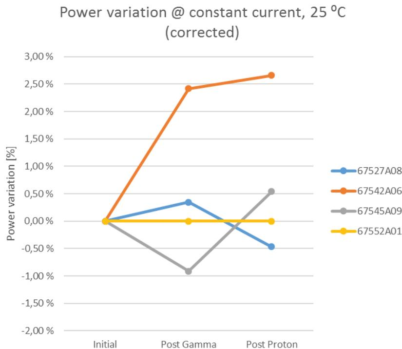
Figure 2-10 The drift in optical power due to radiation environment. The measurements were corrected to account for variation in the test setup. Reference LDM 67552A01, which was not radiation tested, was used for the normalization.
