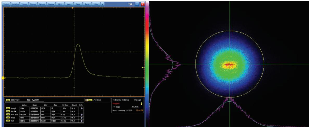
Figure 3. Pulse envelope (left) and far field distribution (right).
