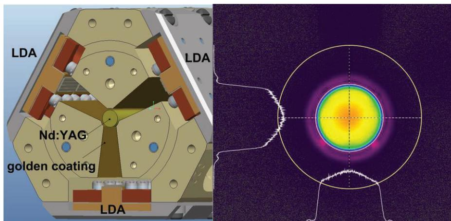
Figure 2. Pump module (left) and gain distribution (right).
