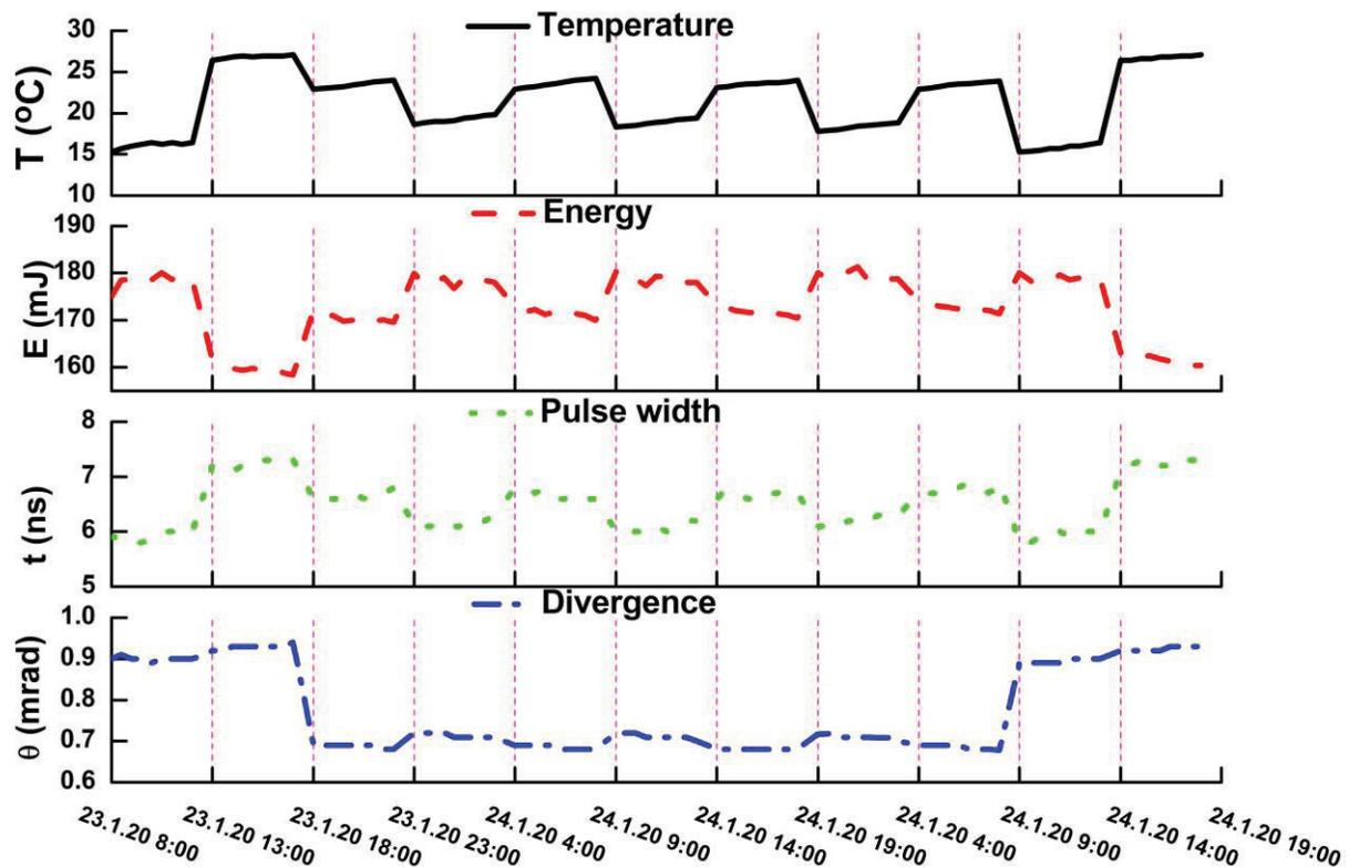
Figure 5. Laser performance during 3.5 thermal cycles in vacuum.
