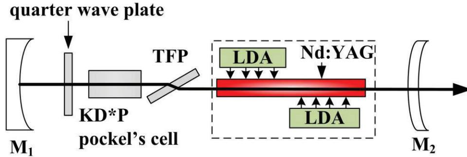
Figure 1. Schematic diagram of the laser resonator.
