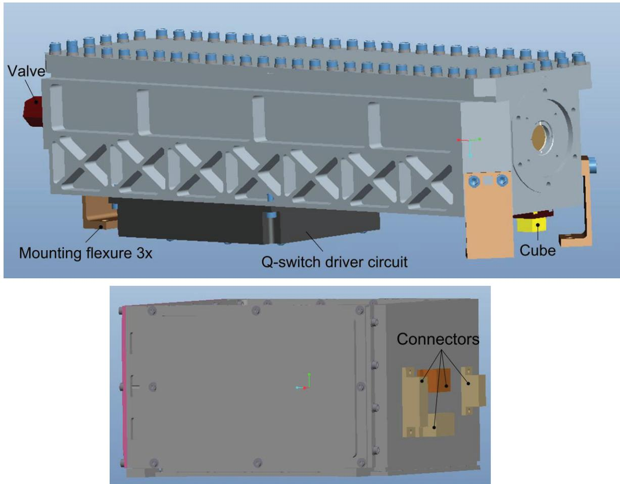
Figure 4. The full laser head (above); laser electronic box (below).
