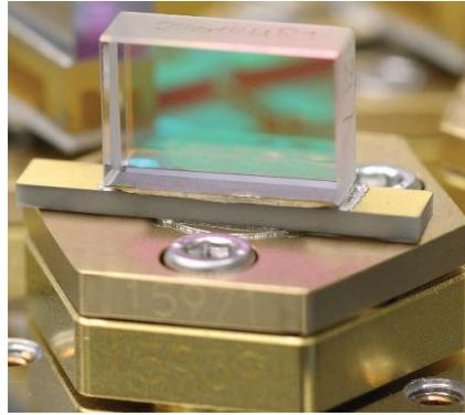
Figure 7. Photo of a basic C-Mount.
