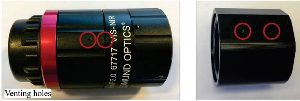
Figure 13. Venting holes drilled in the slit tube (left) and objectives (right) - highlighted in red.
