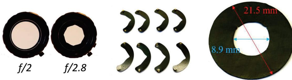
Figure 8. COTS objectives (left) and removed aperture leaves (center). Custom aperture machined (and anodized) for fixed f/2.8 front objectives (right). [credit: M. Hjertenæs]
