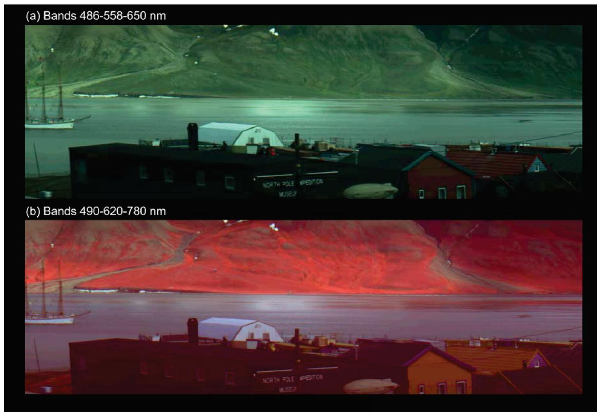
Figure 4. Desktop scan acquired with original HSI design using experimental setup from Figure 2 (right): (a) bands 486-558-650 nm and (b) bands 490-620-780 nm shown for red-green-blue visualization at UNIS, Svalbard.
