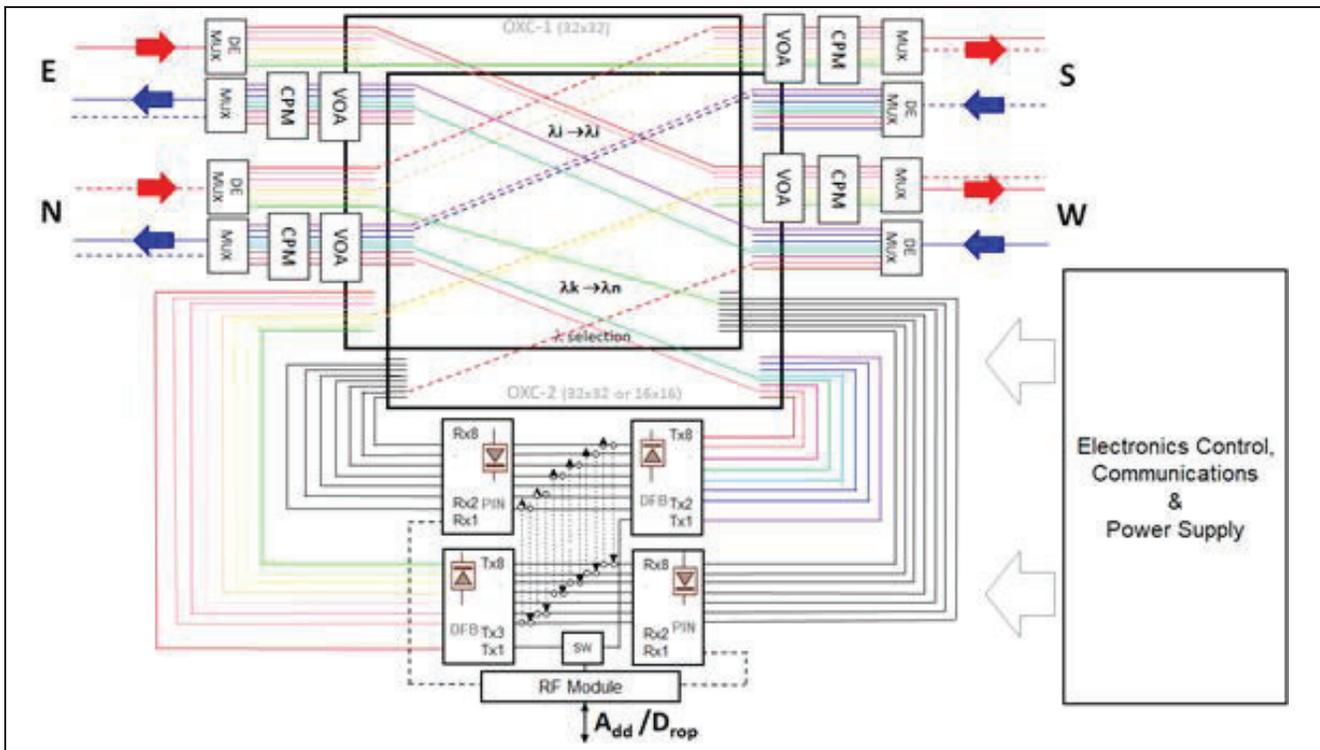
Figure 4. Space ROADM Design- Connection of the channels (wavelengths)
