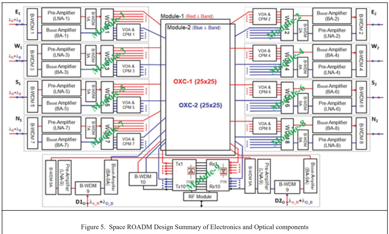
Figure 5. Space ROADM Design Summary of Electronics and Optical components
