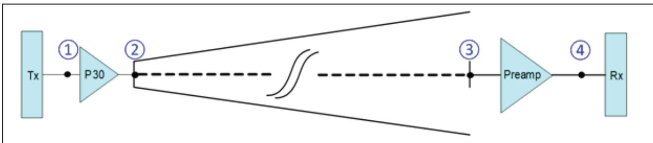
Figure 1. Simplified schematic of an Optical Intersatellite Link (OISL)
