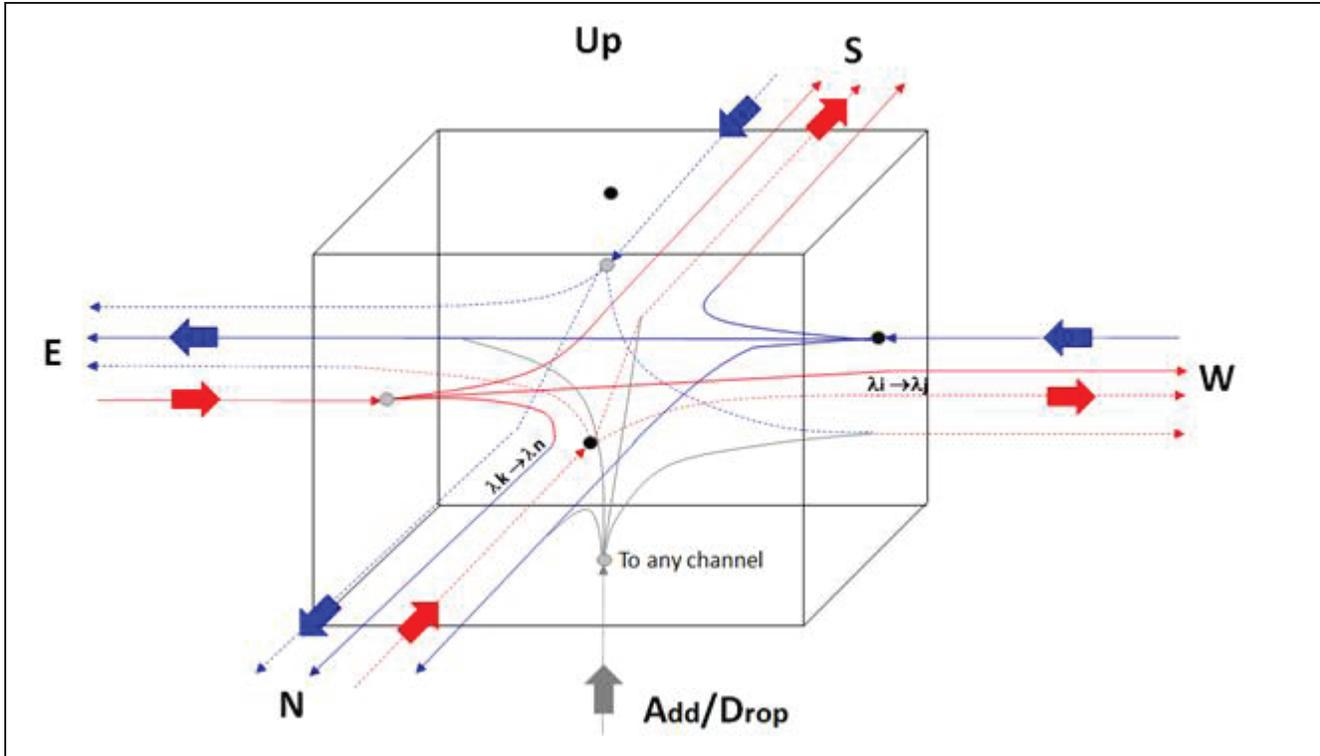
Figure 3. Space Reconfigurable Optical Add-Drop Multiplexer (ROADM) Design
