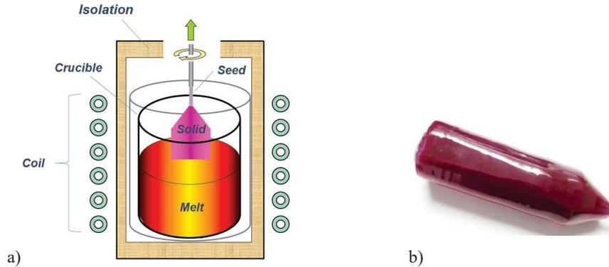
Figure 1: a) Sketch of the Czochralski crystal growth method; b) Example of an Alexandrite crystal boule.
