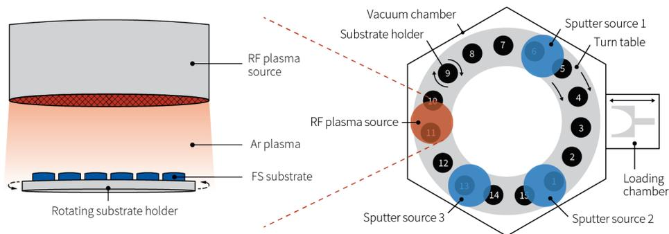
Figure 2: Schematic diagram (left) and ClusterLine RAD sputter platform (right) showing etching procedure.
