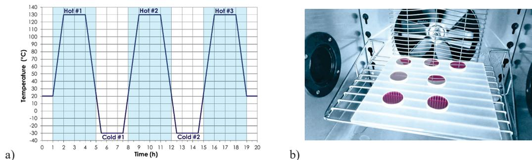
Figure 5: a) Thermal cycling test sequence (schematic); b) Climatic chamber (ESPEC SH-262) for thermal durability tests.
