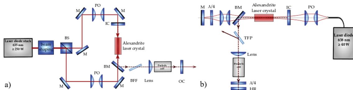
Figure 3: a) high pulse energy - low repetition rate laser demonstrator system; b) low pulse energy - high repetition rate laser demonstrator system. Abbreviations: BS = Beam splitter, M = Mirror, PO = Pump optics, IC = Input coupler, BM = Bending mirror, OC = Output coupler, BFF = Birefringent filter, TFP = Thin film polarizer, HR = Highly reflecting mirror.
