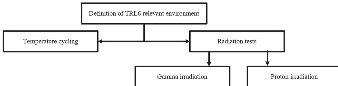
Figure 4: Overview of the planned TRL 6 relevant environmental test campaign within the GALACTIC project.
