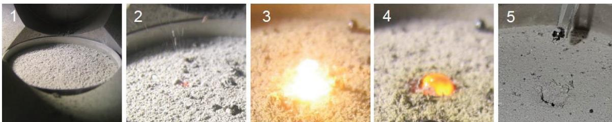
Figure 5. Regolith melting process with the MOONRISE EM: 1. Sample container with regolith simulant, 2. Start of the melting process: some simulant particles are ejected, 3. Melting phase: a sphere of molten simulants forms, 4. Cooling phase: the molten regolith solidifies amorphously, 5. Cooled and solidified sample.
