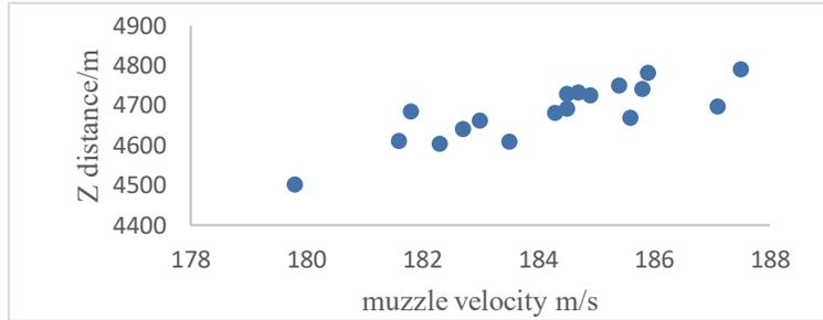
Figure 2. Schematic diagram of the distribution of muzzle velocity - impact point distance.
