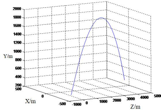
Figure 1. Ballistic curve diagram in the coordinate system of the shooting range.
