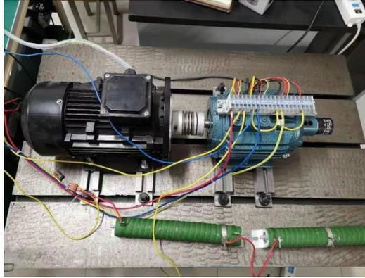
Figure 6. PMSM inverter open circuit experiment platform.
