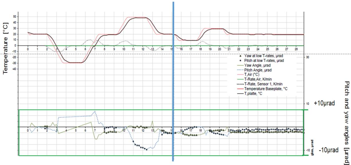
Figure 2-3: Demonstrated angular stability of a soldered opto-mechanical mount
