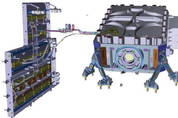
Figure 2-11: Merlin Laser with direct connected radiator
