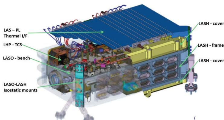
Figure 2-1: Laser concept - Key elements shown at the FULAS demonstrator
