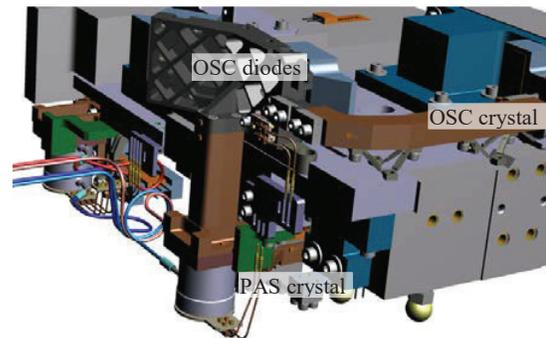
Figure 2-8: MERLIN thermal structure
