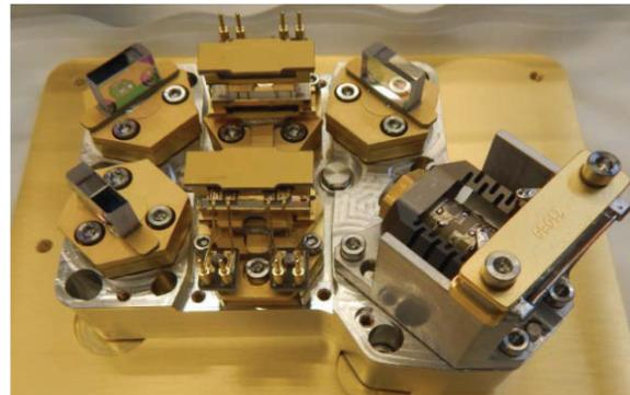
Figure 2-5: MERLIN OPO EQM cavity
