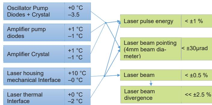
**Figure 2-6:** Overview of thermally induced laser performance sensitivity of the FULAS laser
