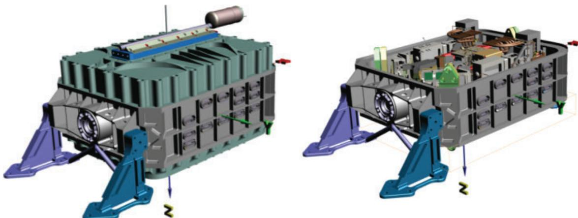
**Figure 2-7:** AEOLUS2 Laser PDR design – left closed housing with payload Loop-Heat-pipe / right open LASH with mounted LASO
