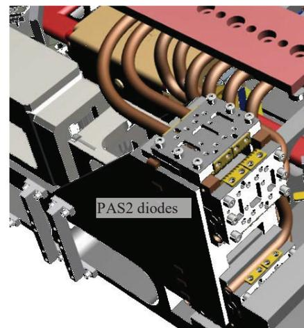
Figure 2-10: ALTA PAS2 pump diode with preliminary routing of Cu\_H2O HP
