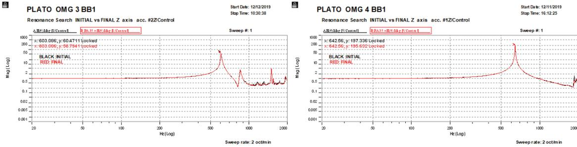
Figure 15. OMG-3 (left) and OMG-4 (right) resonance search comparison
