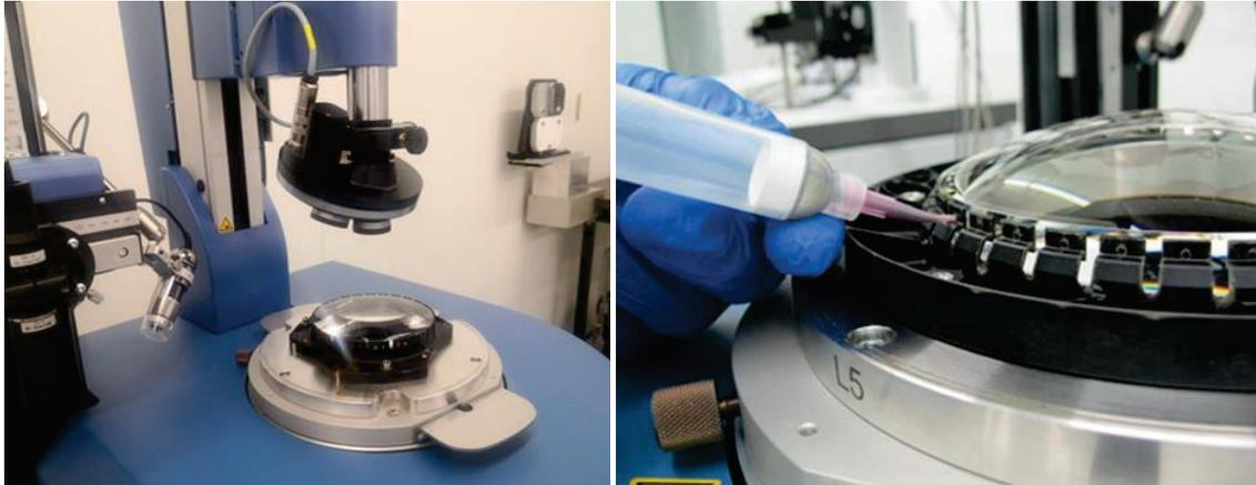
Figure 5. Alignment and bonding of Optical-Mechanical Groups (OMGs) under centering machine.
