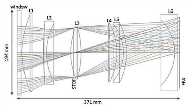
Figure 2. Optical scheme of PLATO Telescope Unit (TOU)
