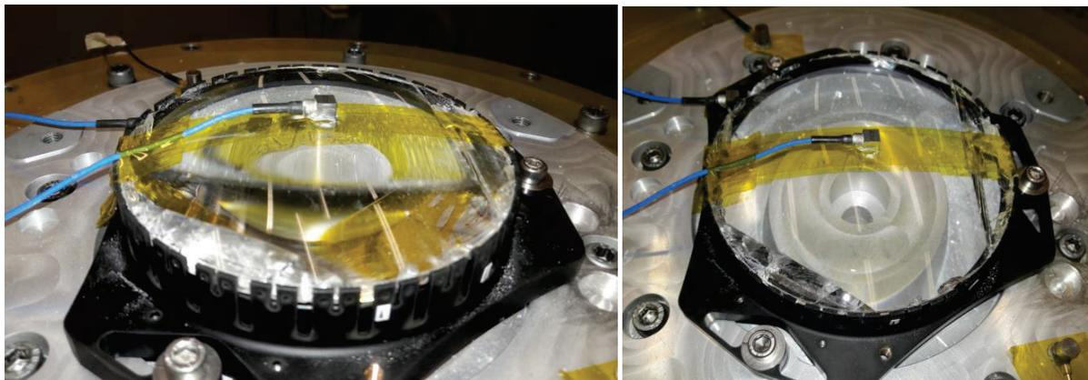
Figure 17. OMG-3 visual inspection after failure.
