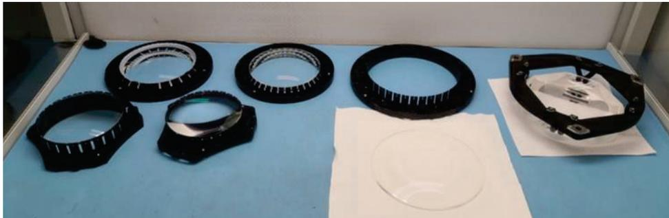
Figure 4. Optical-Mechanical groups (OMGs) of the Telescope
