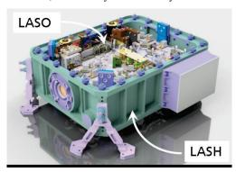
Figure 2 CAD model of laser (LAS): Laser housing (LASH) with integrated optical bench (LASO).
