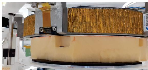
Figure 4. The piezo actuator installed on the elevation arm to inject the external disturbance.
