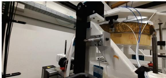
Figure 2. The TS sitting on the safety foam cushion. The yellow disk (coated with kapton) is the aluminum honeycomb RB. Please note the small air gap between the TS and the RB.
