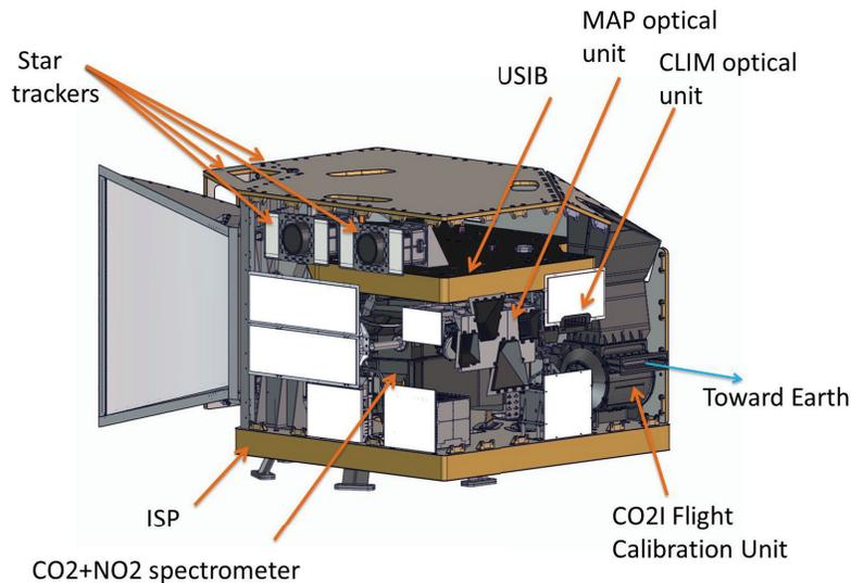
Figure 5. View of the CO2M payload w/o the MLIs (seen from the cold face side, earth toward the right).
