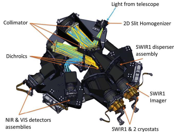
Figure 2. View of the CO2I spectrometer, that uses a 2D slit homogenizer and collimator common to all the bands to provide native quasi-perfect co-registration, dichroics to split the 4 bands into dedicated spectrometer bands with high efficient gratings, imagers with limited number of lenses to limit the straylight, and detectors. The spectrometer is assembled onto an optical bench whose rigidity and stability is ensured by the adequate use of Si3N4 ceramic.
