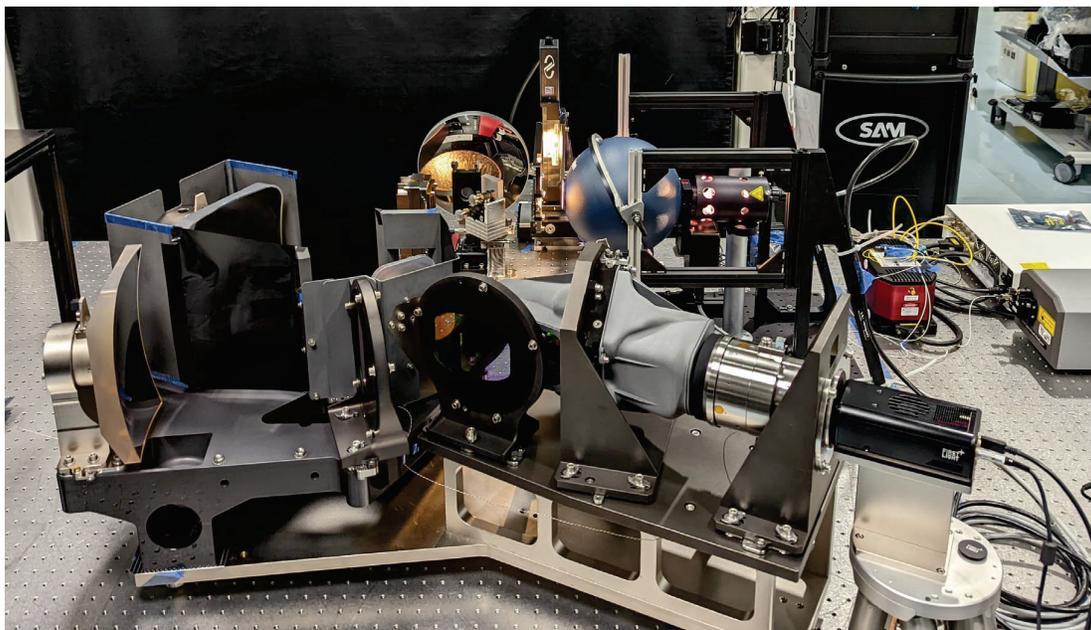
Figure 6. Partial view of the EBB. The collimator assembly can be seen on the left side, 2 of the 3 dichroics at the center, and the SWIR-1 assembly (disperser under its light grey baffles, imager in its barrel, GSE camera) on the right.
