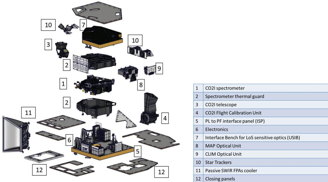
Figure 4. Structuration of the payload, with the CO2I spectrometer at its core.
