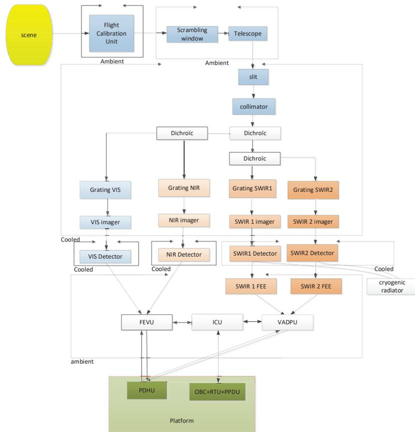
Figure 1. CO<sub>2</sub>I functional architecture, that includes the NO<sub>2</sub> band. The core of the instrument is the spectrometer, that features a single slit and collimator for nominal co-registration, and dedicated gratings and imagers for nominal radiometric performances.
