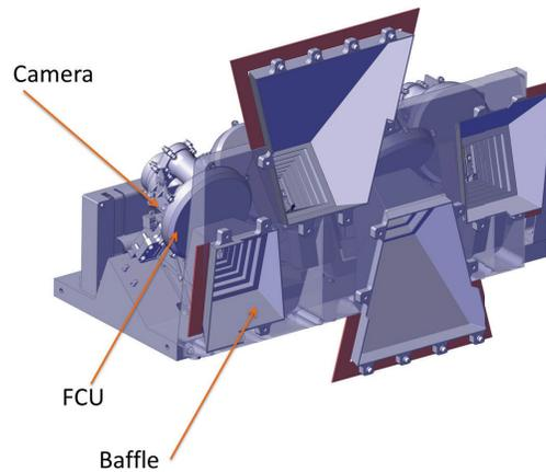
Figure 3. view of the MAP Optical Unit (covers and structure removed), showing the modular use of identical cameras to cover the specified along-track field of view.
