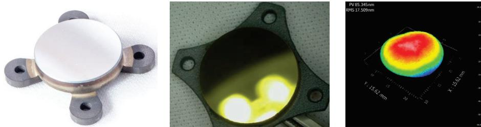
Figure 2. Mirror type 1 & silver coating (left), type 2 & gold coating (middle), and RWE tests after integration (right)
