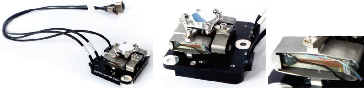
Figure 3. PFSM-150S Engineering Model (left) & Strain Gauge onto piezo ceramic (right)
