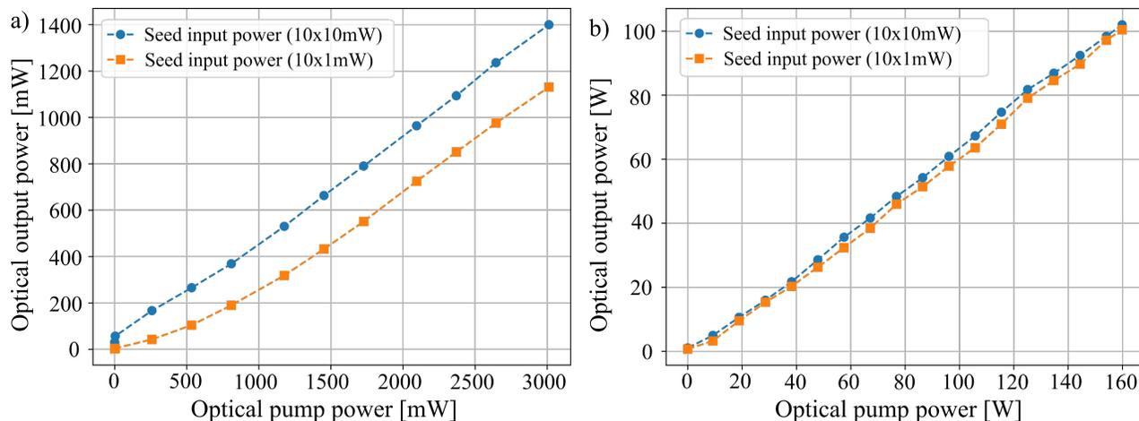
Figure 4: Optical slope at different injected optical pump powers of the pre-amplifier in a) and of the main-amplifier in b). The performance was tested with seed input powers of 10 mW and 1 mW per channel.
