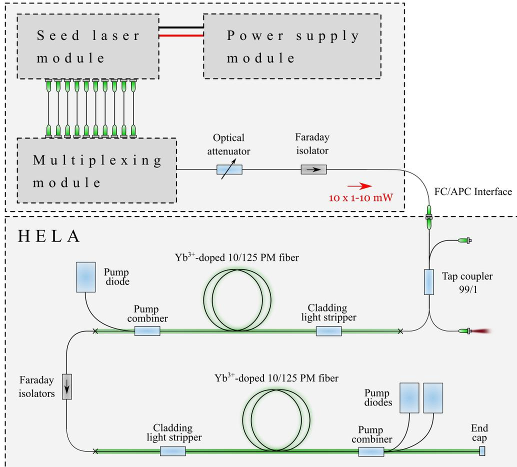
Figure 1: Setup of the HELA design based on a two-stage amplifier architecture including in-house manufactured fiber components. A corresponding seed laser system with 10 optical channels guided inside a single-mode fiber was developed in order to demonstrate the capabilities of the amplifier system.
