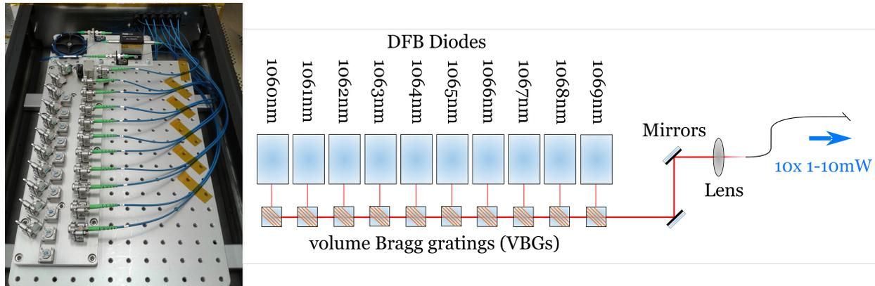
Figure 2: Concept of the HELA seed laser system based on volume Bragg gratings and a free-space coupling into a polarization-maintaining single-mode output fiber.
