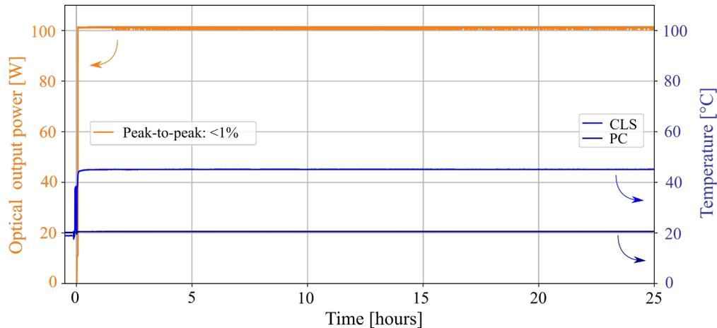
Figure 6: Long-term measurement of the optical output power of the HELA system in orange. The temperatures of the key components of the main amplifier (CLS: cladding light stripper, PC: pump combiner) are shown in blue.
