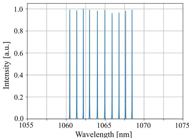
Figure 5: Optical spectrum after the main-amplifier at a total output power level of 100 W (10x10mW of seed input power).
