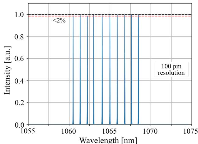
Figure 3: Optical spectrum of the 10 seed laser channels with peak-to-peak power variations <2%.
