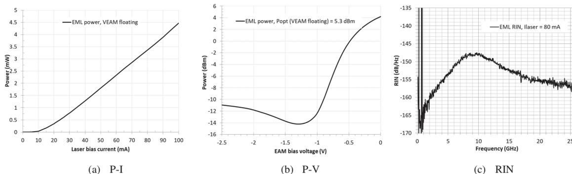
Figure 2. EML characteristics at room temperature (chip set @45°C)
