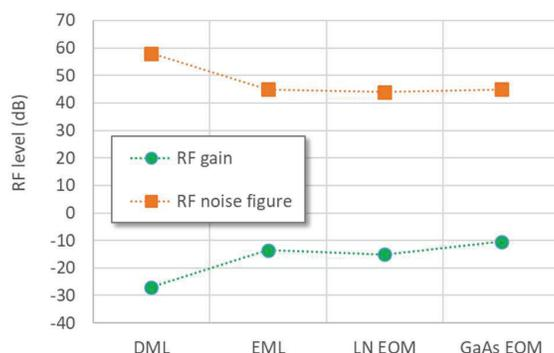
Figure 10. RF gain and noise figure of photonic frequency up-converter using various photonic RF transmitter types
