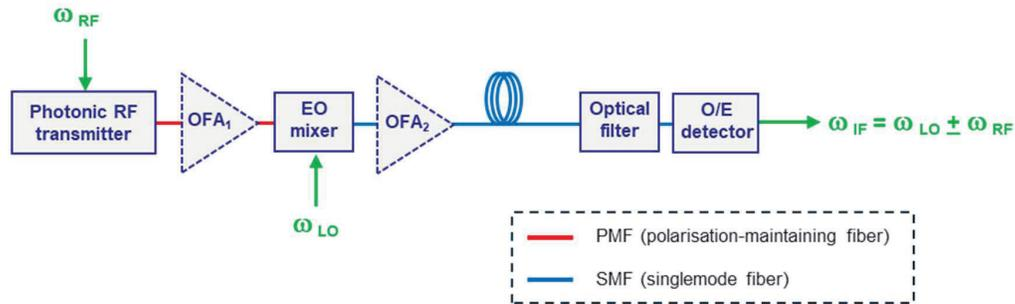
Figure 8. Reference configuration for photonic RF frequency conversion
