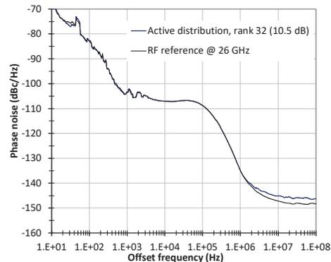
Figure 7. RF phase noise for active EML-based LO distribution at 26 GHz
