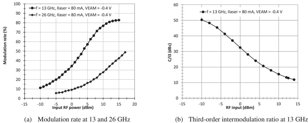
Figure 3. EML RF-characteristics at room temperature (chip set @45°C)
