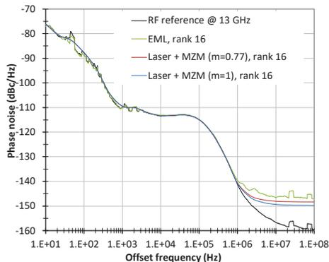
Figure 6. RF phase noise of Active LO distribution at 13 GHz for an EML (measurement) and Laser + MZM (simulations)
