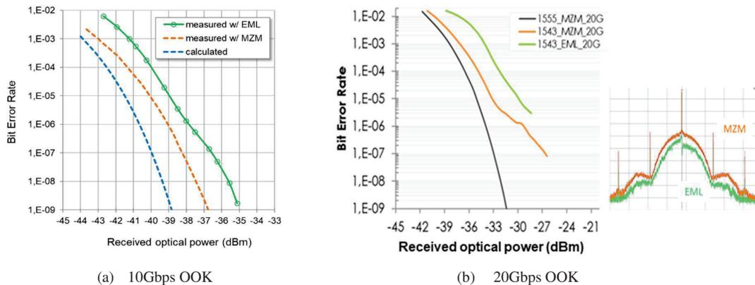
Figure 12. Results of digital transmission experiments using EML and comparison with reference MZM-based transmitter
