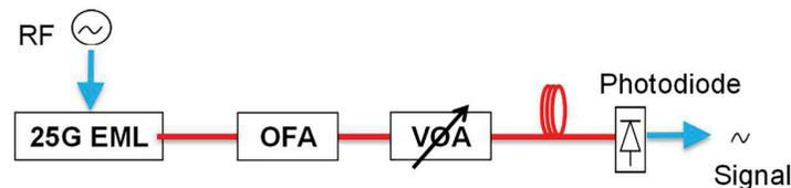
Figure 4. Schematic of the optical LO distribution set-up
