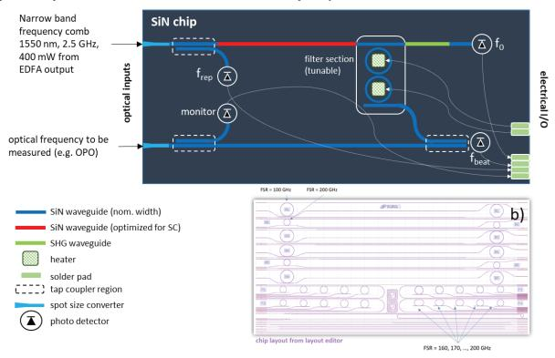
Figure 5. a) Schematics of a SiN based frequency detector:  $f_{rep}$  – pulse repetition rate / comb spacing,  $f_{beat}$  – heterodyne beat frequency between comb and instrument (e.g. OPO/OPA output),  $f_0$  – Offset frequency b) Design outline of the SiN test chip that has been manufactured for parameter optimization and radiation testing.
