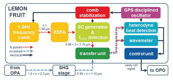
Figure 2. Overall outline of the LEMON frequency reference unit (FRUIT) with the main interfaces to the other instrument subunits. EDFA: erbium doped fiber amplifier, SC: super continuum, OPA: optical parametric amplifier, being the last amplification stage of the main laser, SHG: second harmonic generation, OPO: optical parametric oscillator, being the first element of the main laser that generates the spectroscopic laser pulses.
