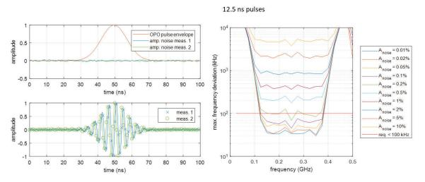
Figure 1.Simulation of resolution limits for heterodyne beat note detection: The upper left panel shows the envelope of the OPO-pulse and the noise contribution. The lower left panel gives two examples of simulated beat signals. The right panel provides the results. The detailed explanation can be found in the text.
