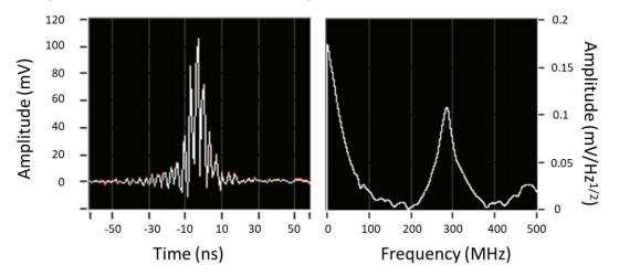
Figure 4. Beat Signal obtained between the FRUIT and pulsed laser @ 1064 nm. Left hand side: The transient beat signal as detected with the 1 GHZ analogue-digital-converter (ADC) – 1 Sample = 1 ns. Right hand side: Fourier analysis of the same signal for retrieving the centroid of the offset frequency between the known comb mode and the laser pulse.
