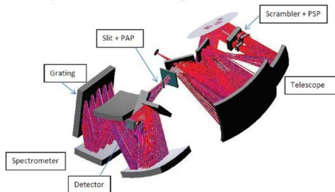
Figure 1. Optical design of MicroCarb instrument
