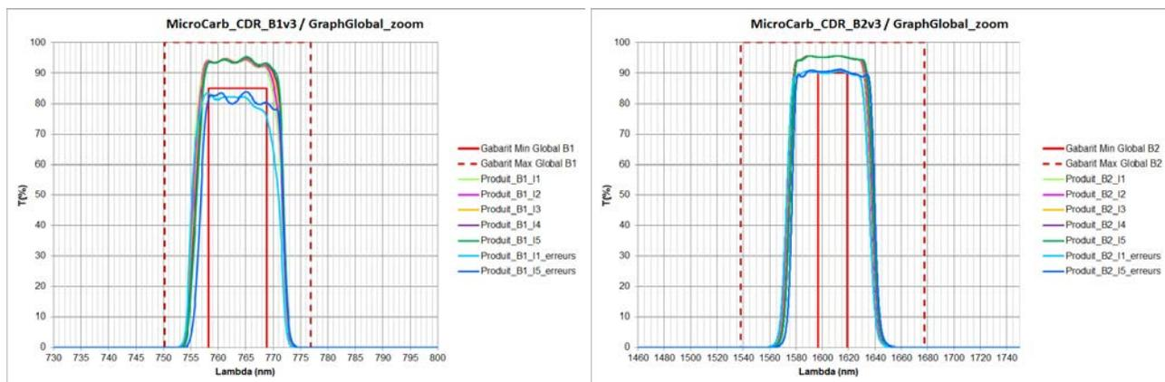
Figure 3. Global performance in transmission of B1 (left) and B2 (right) channels
