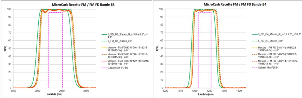
Figure 9. Performance in transmission of B3 (left) and B4 (right) Detector Filters flight models.
