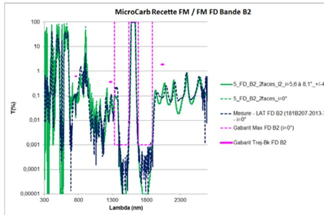
Figure 10. Performance in transmission (log scale) of B2 Detector Filter.
