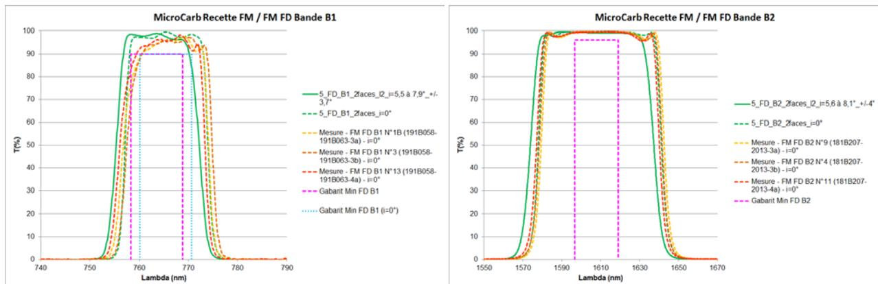
Figure 8. Performance in transmission of B1 (left) and B2 (right) Detector Filters flight models.
