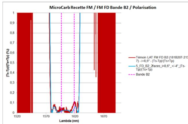
Figure 11. Polarization sensitivity of B2 Detector Filter.
