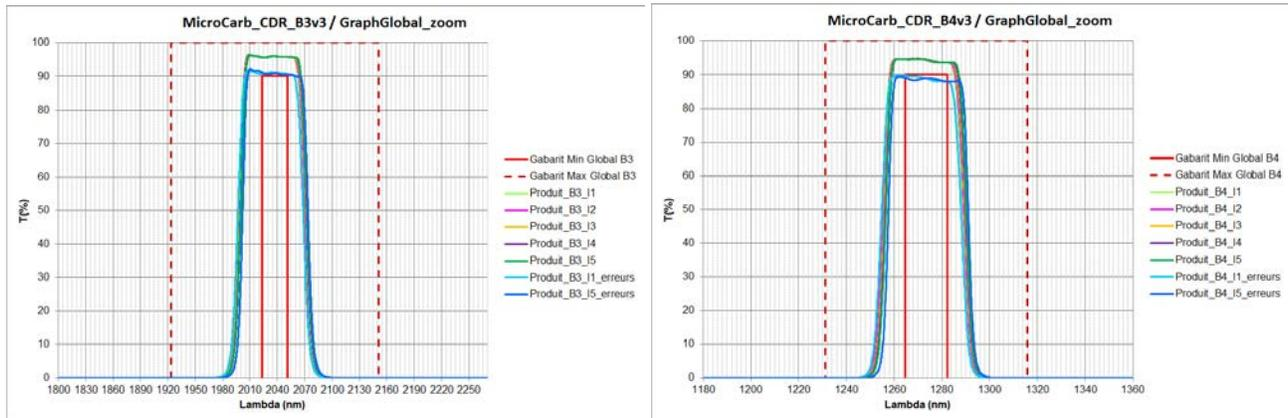
Figure 4. Global performance in transmission of B3 (left) and B4 (right) channels
