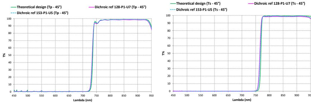
Figure 13. Spectral response measurements at 45° angle of incidence, in P (left) and S (right) polarization in [450-950nm] spectral range of two dichroic beamsplitters manufactured with PIAD coating technology.
