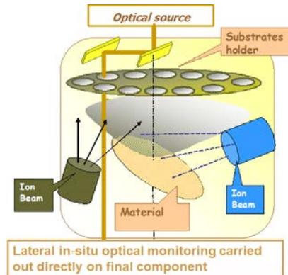
Figure 7. Dual Ion beam sputtering principle
