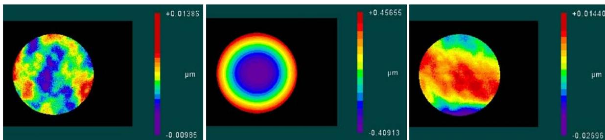
Figure 14. Flatness measurement after polishing (left), after dichroic coating on front face (center), after dedicated antireflection coating on rear face (right).
