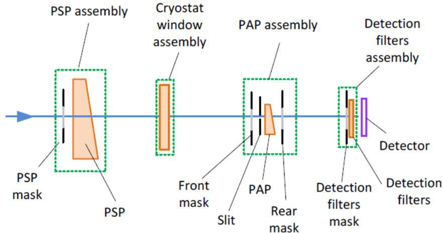
Figure 2. Sketch of the Microcarb optical path
