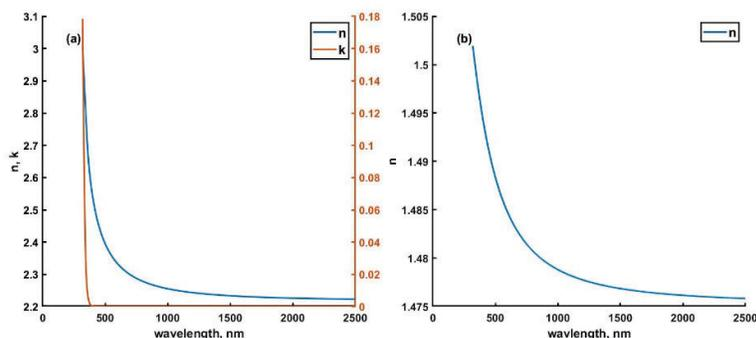
Figure 4. Refractive indices of Nb<sub>2</sub>O<sub>5</sub> (a) and SiO<sub>2</sub> (b).
