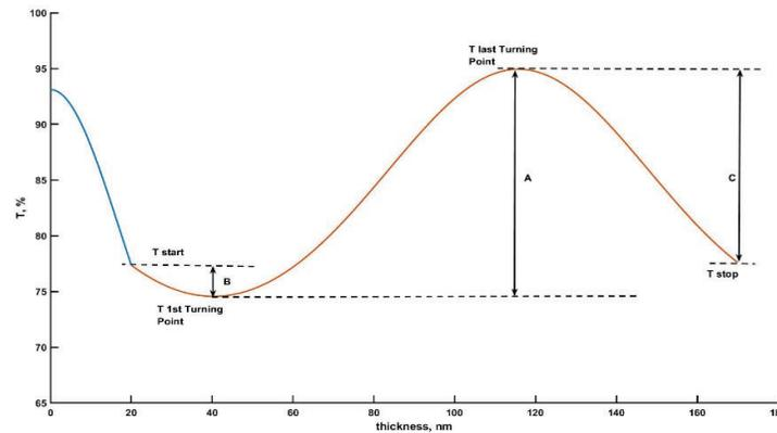
Figure 1. Transmittance evolution versus thickness or ‘monitoring curve’ of 20 nm Nb<sub>2</sub>O<sub>5</sub> layer – blue curve, followed by 150 nm SiO<sub>2</sub> layer -red curve, Monitoring wavelength 450 nm. A – total amplitude – difference between turning points (or maximum and minimum of monitoring signal); B - start amplitude – difference between start transmittance and first turning point; C – final amplitude – difference between last turning point and trigger point.
