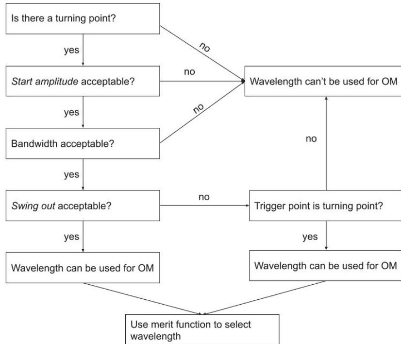
Figure 3. Flowchart of the monitoring wavelength selection process.
