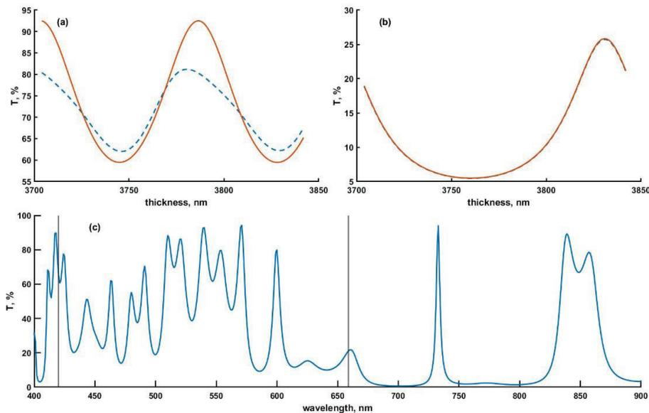
Figure 2. Monitoring curves, solid line represents theoretical monitoring curve, dashed line represents theoretical monitoring curve if bandwidth is 3 nm. (a) the monitoring wavelength is 420 nm, (b) 659 nm, (c) spectral performance at the end of the layer, vertical lines are plotted at 420 and 659 nm.
