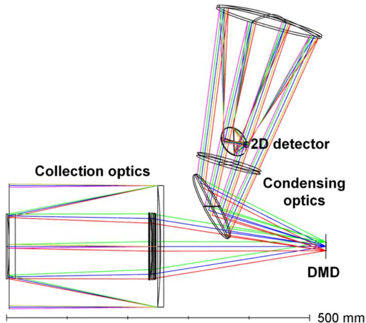
Figure 4. SISSI instrument 3D optical CAD.
