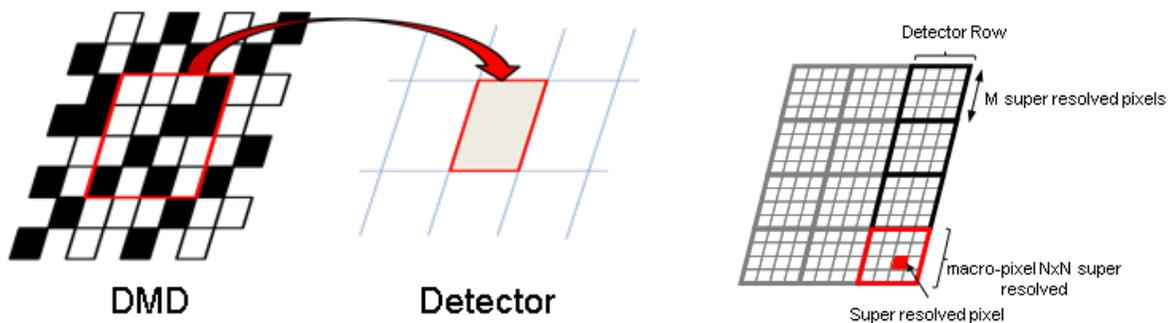
Figure 1. Super resolution for SISSI instrument: macro-pixel, and micro-pixel
