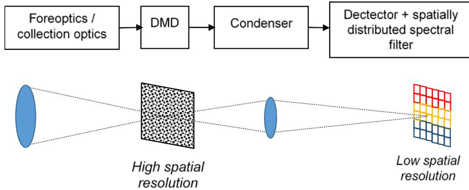
Figure 3. Functional blocks of SISSI instrument optical section
