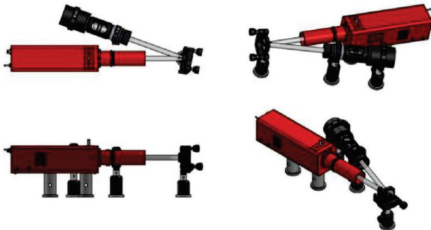
Figure 5. Design of the reflectometer's equipment for the measurements of reflective properties.
