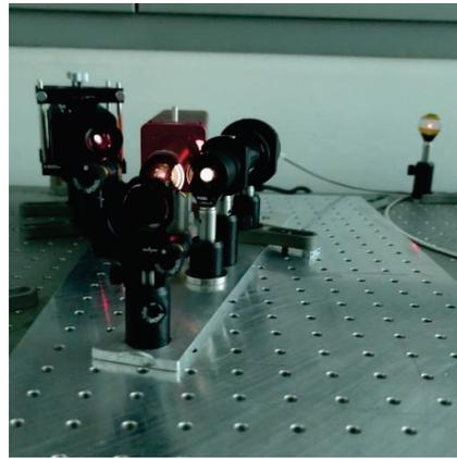
Figure 7. Picture of the lab setup with the laser input switched on (left), the target of the laser (right) and a stage in front of the sensor.
