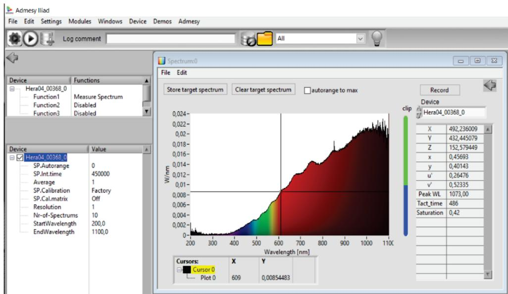
Figure 8. Spectrum of the irradiance read by the spectrometer using Admesy Iliad® software.
