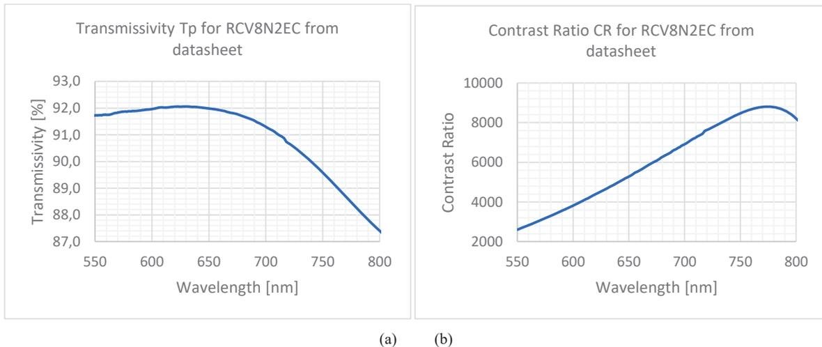
Figure 3. Properties of transmissivity  $T_p$  and Contrast Ratio CR of polarizer RCV8N2EC from its datasheet.
