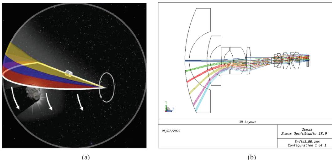
Figure 1. In (a) schematics of the acquisition of the comet and the full sky through the spinning motion of B2. In (b) ray tracing through the EnVisS optical head performed in Zemax® [3].
