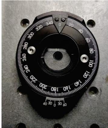
Figure 6. Rotator stage with the polarizer inside.
