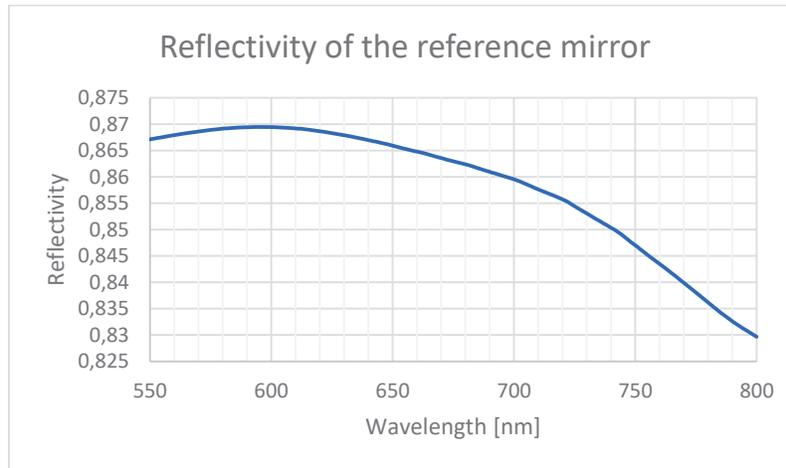
Figure 9. Reflectivity of the reference mirror.
