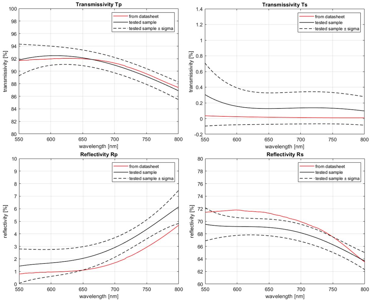
Figure 10. Results of lab tests for the characterization of the polarizer and comparison with data from the supplier; the optical parameters shown are transmissivity  $T_p$  and  $T_s$  and reflectivity  $R_p$  and  $R_s$ .
