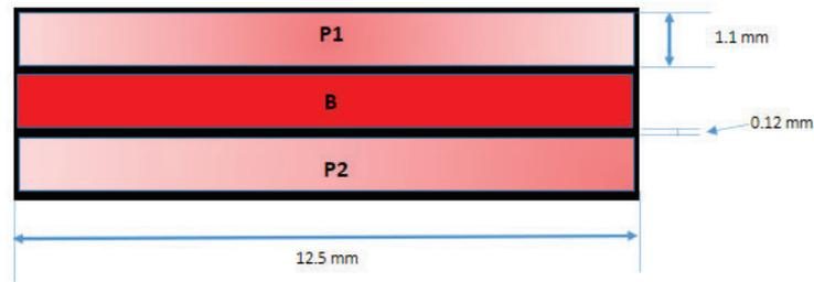
Figure 2. Schematic design of the filter assembly: a central broadband (B) filter and two linear polarizers (P1 and P2) at the sides. The useful filter areas dimensions are highlighted, the remaining of the filter assembly will be black coated.
