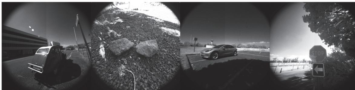
Figure 15: Examples of raw images acquired by the custom SFA. Vignetting is due to the optical system used for data acquisition (aperture  $f/4$ ) and is corrected during image processing (through a flat field) after dark signal subtraction.
