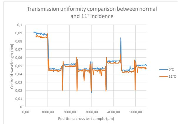
Figure 8: transmission uniformity across sample, for normal collimated incident light (blue), and for collimated 11° tilted incident light (orange)
