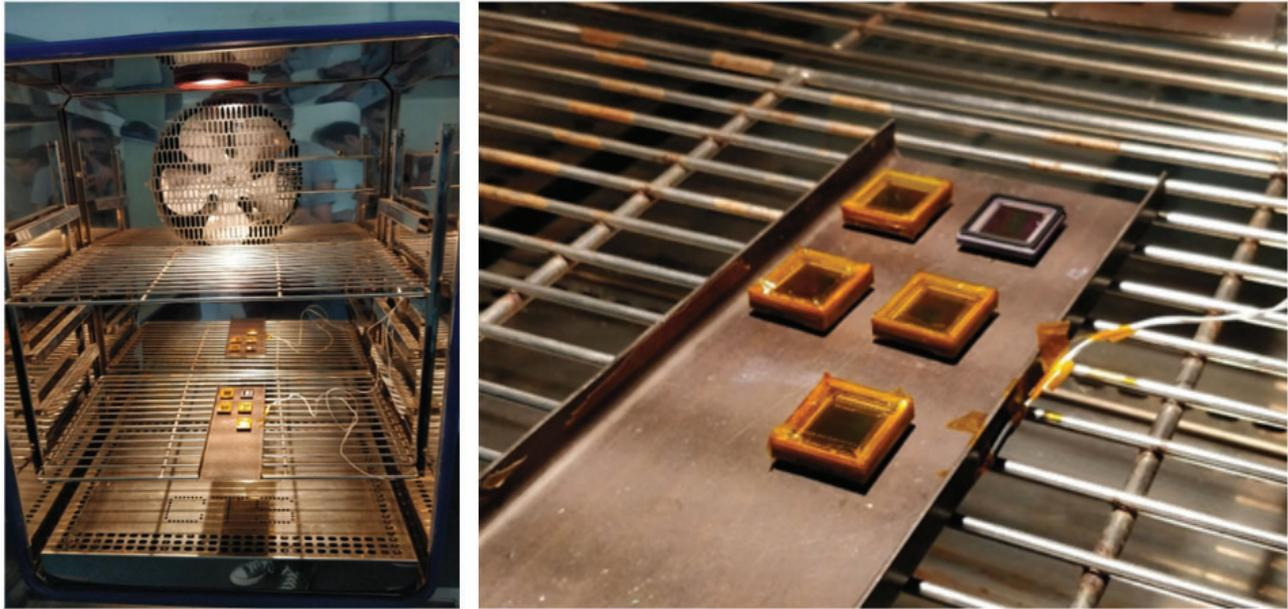
Figure 2. Picture of curved image sensor samples inside the thermal chamber
