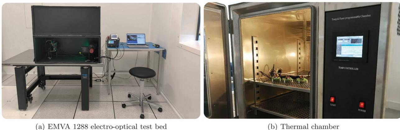
Figure 1. CIS characterization test beds and environmental test equipment
