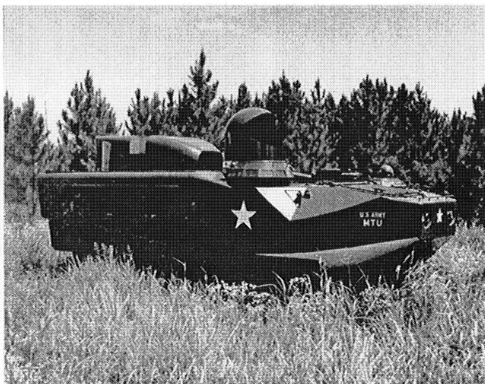
Fig. 19. MTU vehicle with mockup of the beam director turret and heat exchangers. The vehicle is a Marine vehicle, which caused the Army some heartburn.
