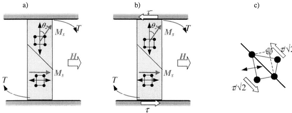
Fig. 4. a) Schematic of twinned Ni-Mn-Ga martensite crystal constrained against the clockwise torque,  $T$ , induced by application of a magnetic field. b) The constraint applies a counterclockwise shear couple to the sample to maintain equilibrium. c) Schematic of twinned unit cell straddling the twin boundary. The component of the constraining shear across the twin boundary promotes growth of the field-favored variant.
