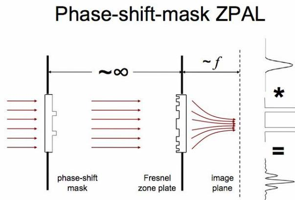
Figure 4: Schematic of a ZPAL phase-shifting strategy that would produce narrower peaks in the point-spread function, at the expense of higher sidelobes. This would be useful in exposing isolated lines or spaces but generally not for patterns of arbitrary geometry.
