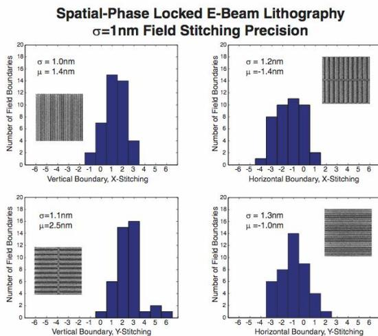
Figure 1. Histograms of field-stitching errors obtained with real-time spatial-phase locked e-beam lithography (global grid mode). Both x- and y-stitching errors are shown for the horizontal and vertical field boundaries. The mean and standard deviations are given on each histogram. We believe that intrafield distortion (which was corrected in software) was a limiting factor in these results.
