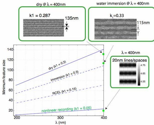
Figure 5: Plot of the minimum feature size versus wavelength for ZPAL. Experimental results associated with exposure in air and in water immersion [10] are indicated and shown in micrographs. Simulation results are shown for the non-linear recording for which feature size of  $\lambda/20$  is predicted.
