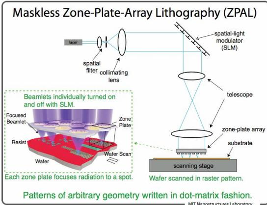
Figure 2: Schematic of the Zone-Plate-Array-Lithography (ZPAL) system. The spatial light modulator is an array of 1024 grating-light valves from Silicon Light Machines, the light source is a 400nm-wavelength GaN laser, the zone plates of the array are phase zone plates fabricated using SEBL and HSQ resist. The stage is moved under computer control enabling patterns of arbitrary geometry to be written in a dot-matrix fashion.
