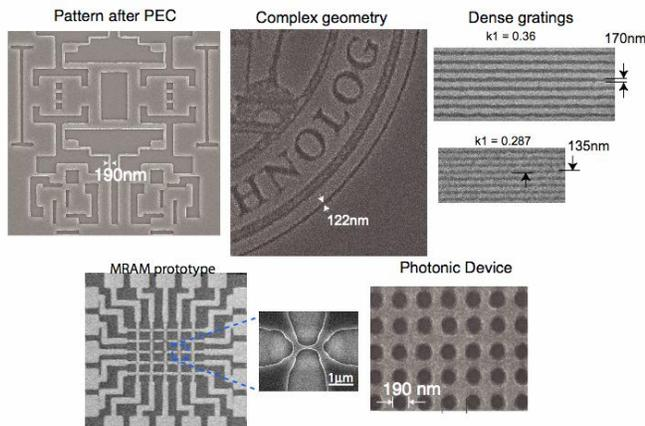
Figure 3: Experimental results obtained with the ZPAL system at MIT. From upper left clockwise: pattern written with proximity-effect correction (PEC); portion of the MIT seal with 122nm linewidth; dense lines and spaces written with  $k_1$  as fine as 0.287; upper level of a 2-level magnetic random access memory prototype; magnified view showing the overlay of the upper level on the lower-level magnetic ring; portion of a 2D photonic crystal device pattern.
