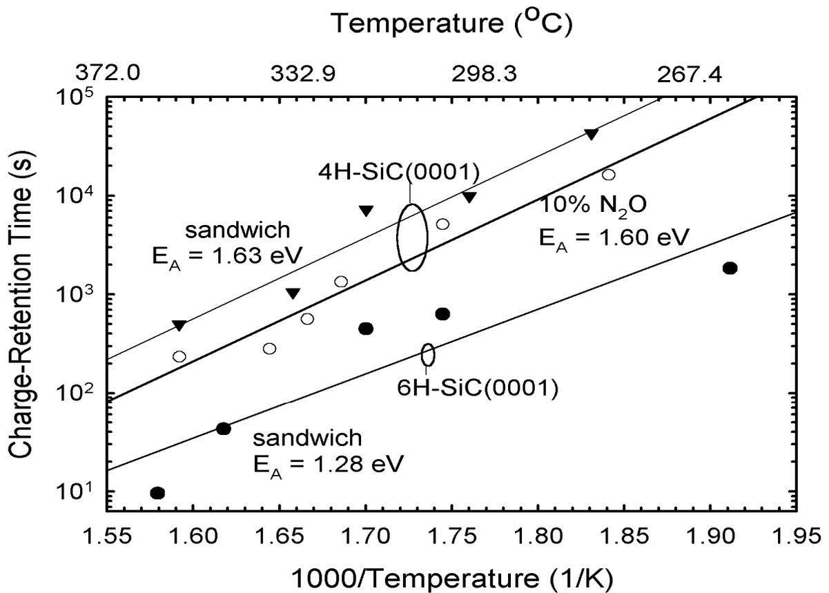
Figure 2 Retention of Non equilibrium Charge in SiC MOS Capacitors
