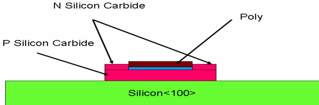
Figure 3 Schematic of single transistor memory cell
