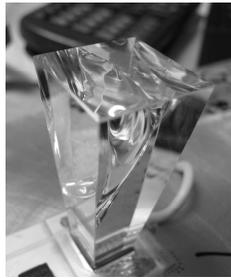
Fig. 10a. Glass type A fractured
