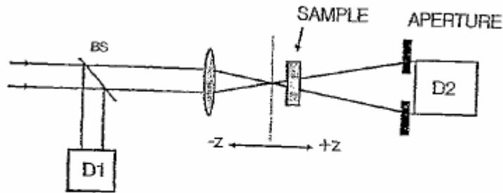
Figure 2. Z-Scan Technique from Ref. 16 figure 4. Note that the sample is scanned through the beam focus. The ratio of the readings of D1 and D2 is measured. The fit from the curve of this ratio vs. Z (position relative to the focus) give the nonlinear index of refraction. If the aperture (D2) is fully open and captures all the transmitted beam then nonlinear absorption is measured.
