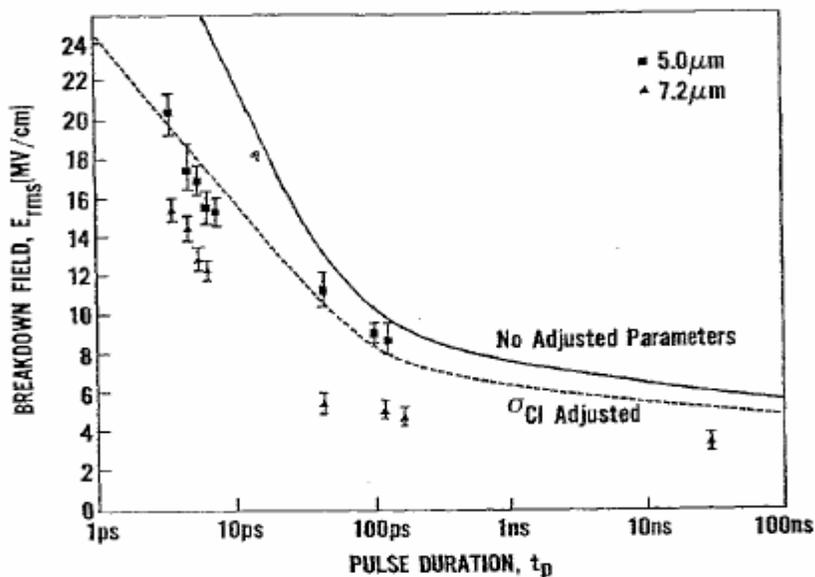
Figure 7. The RMS breakdown field data for NaCl (78-NC-6) at 1.06  $\mu\text{m}$  are plotted as a function of pulse duration,  $t_p$ . The solid line and dotted line were obtained from the theory developed by Sparks et al. [28] for NaCl at room temperature. The dotted line uses a different value for the absorption cross section for Cl ions in the theory than the solid line.
