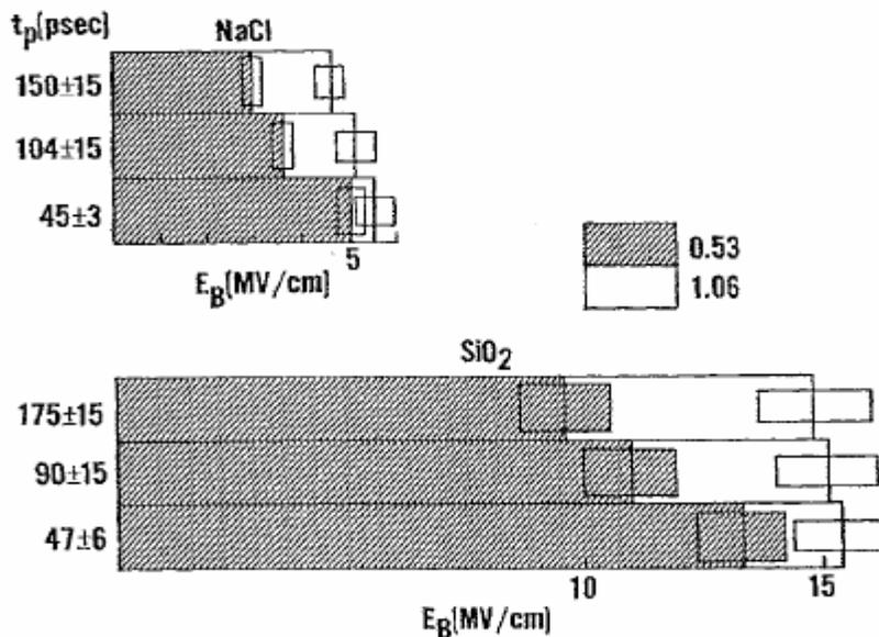
Figure 8. Wavelength dependence of the breakdown field  $E_B$  for NaCl and SiO<sub>2</sub> for a variety of laser pulse widths. All the above data was taken on the same sample of NaCl and the same sample of SiO<sub>2</sub>. The 1.06  $\mu\text{m}$  thresholds are taken from Ref. 2 and are interpolated from measurements made at spot size 6.1 and 10.3  $\mu\text{m}$ .
