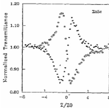
Figure 4. This is figure 6 from ref. 16 and it shows the power of the Z-Scan technique to help understand relevant nonlinear interactions, including 2PA, excited state absorption (free carrier absorption), and nonlinear refraction for ZnSe at 0.53 microns and 30 psec pulses. The bottom curve shows the results of increasing the irradiance by about a factor of 5, and the fit is excellent indicating that the essential physics is accounted for in this measurement.
