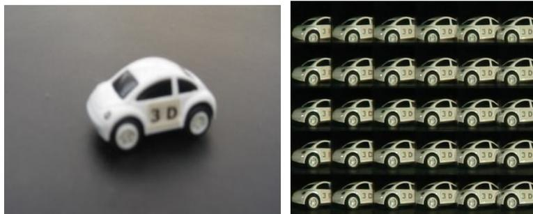
Fig. 3. (a) A sample car object used in our experiments (b) Cropped sets of 6x5 integral images of one of the cars used in the experiments. Each elemental image is composed of 73 x 73 pixels.
