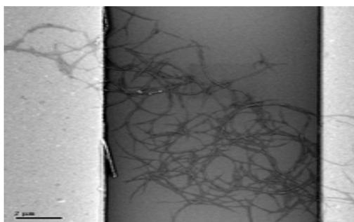
Fig. 2.0-2 Single sensor element with carbon nanotubes across gold electrodes
