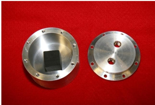
**Fig. 3.2-1** Propellant Aging Sample in Aging Cup
