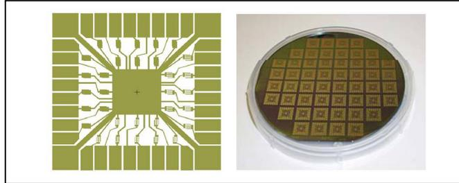
**Fig. 2.3-1** Details of sensor elements (left) and chip/wafer (right)
