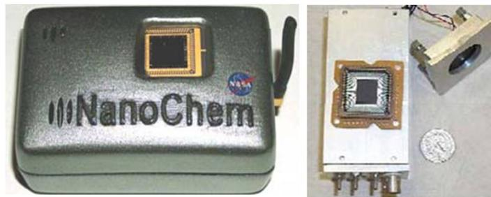
**Fig. 2.3-2** Complete NASA-Ames SWCNT sensor package
