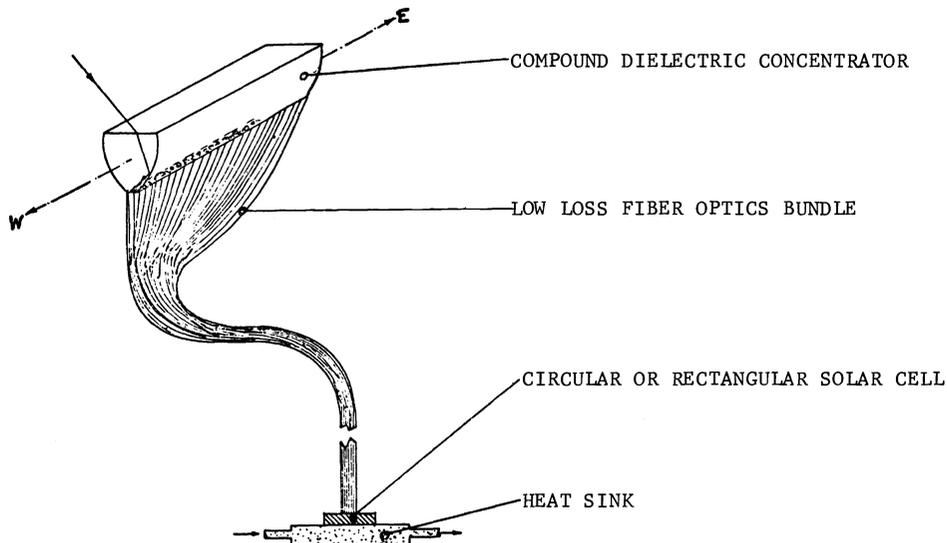
Figure 15. Compound dielectric concentrator coupled to solar cell for geometrical matching and heat isolation purposes.
