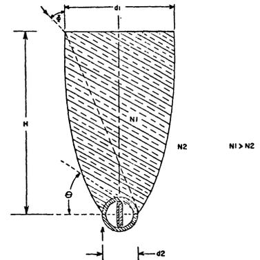
Fig. 13. DCPC with vacuum insulated absorbing element.
