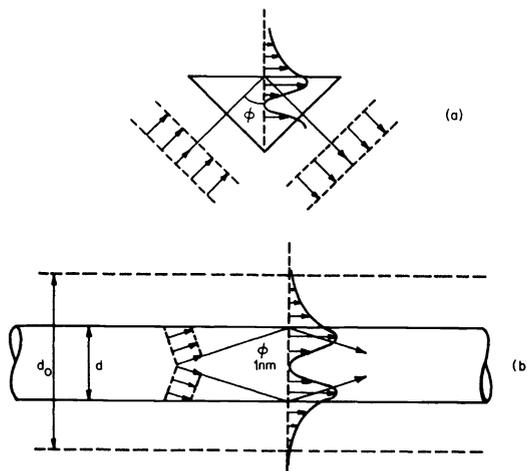
Figure 3. Electric field strength for total internal reflection at a) plane boundary, b) cylindrical boundary.
