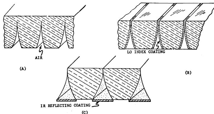
Figure 11. Various configurations of the dielectric compound parabolic concentrator.
