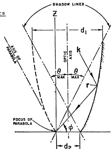
Fig. 9. Compound parabolic concentrator cross-section.
