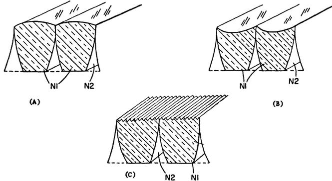
Figure 12. DCPC with various entrance aperture modifications.
