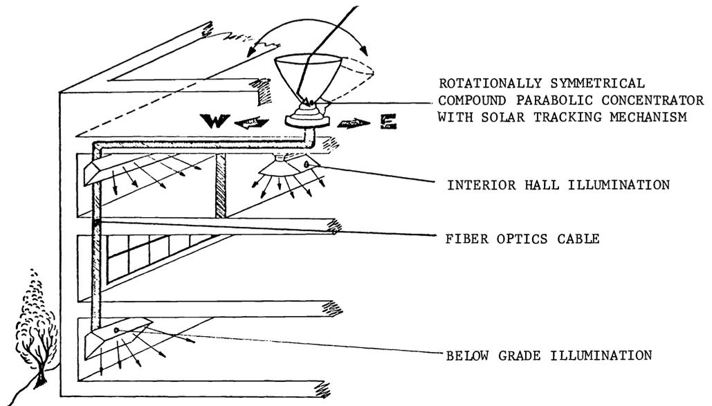
Figure 16. Tracking solar concentrator used with low loss fiber optics to illuminate the interior portions of buildings.
