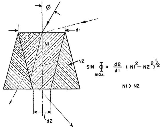
Figure 6. Dielectric total internal reflection concentrator diagram.
