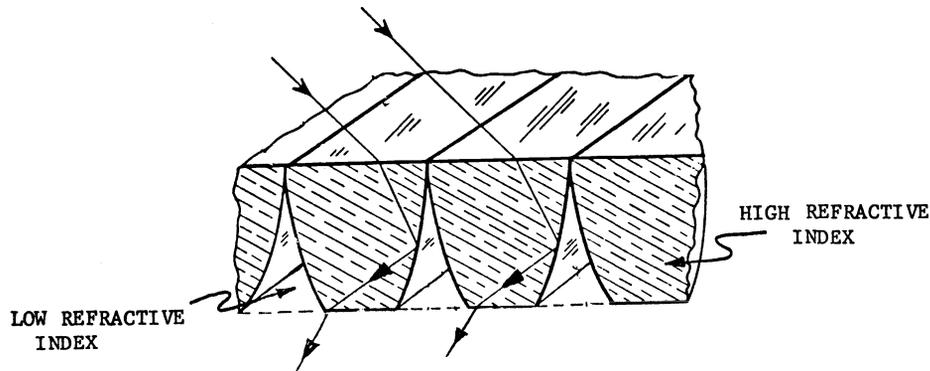
Figure 10. Diagram of dielectric compound parabolic concentrator.
