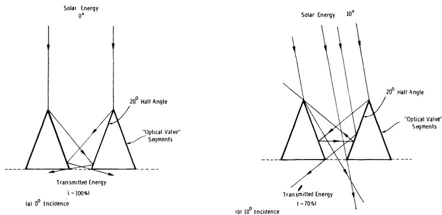
Figure 7. Path of normal incidence rays (a), and rays inclined at 10° (b), through the optical valve.
