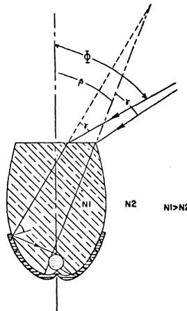
Figure 14. Partial TIR compound elliptical concentrator.
