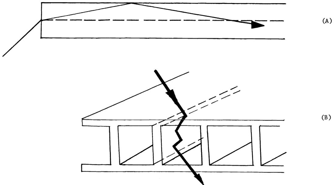
Figure 4. Solar collector window with optical ribs, (A) illustrating the conduction of solar radiation by total internal reflections and (B) a window with optical rib.
