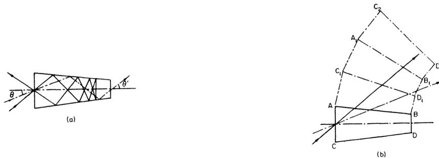
Figure 5. Ray passage along a reflecting wedge: (a) Illustrating the limiting ray and the returning ray passage; (b) Geometrical construction used for calculating the acceptance angle of a reflecting wedge.
