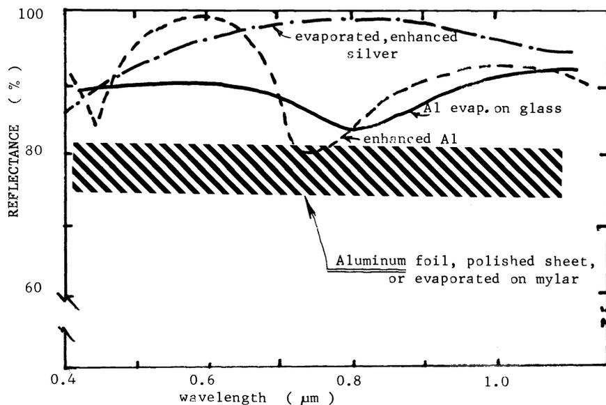
Fig. 1. Spectral reflectivity of various types of metallic reflectors.
