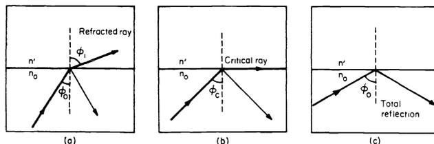
Figure 2. Ray incident at a plane interface between a high and low refractive index medium when (A) the ray is refracted (B) the ray traverses along the interface and (C) total internal reflection occurs.
