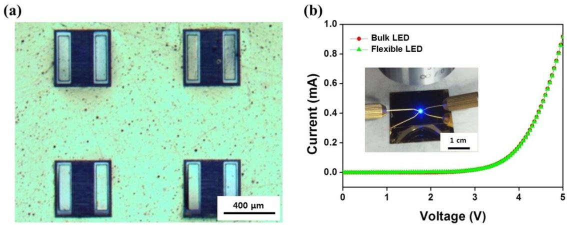
Figure 5. (a) Optical Image of GaN LED arrays on flexible substrate (b) I-V curve comparison between Bulk LED and Flexible LED
