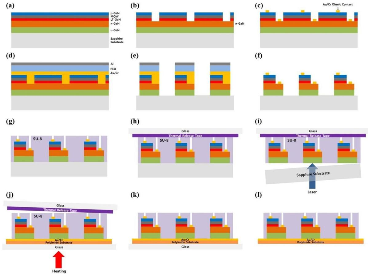
Figure 3. Schematic diagrams of the fabrication of high quality flexible GaN LED arrays from sapphire substrate.
