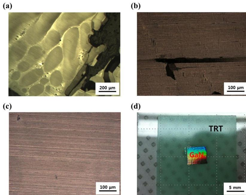
Figure 2. Optical Images of laser lift offed surface on different carrier substrates (a) on PDMS stamp (b) TRT (c) TRT with SU8 passivation. (d) photograph of the sample (c)
