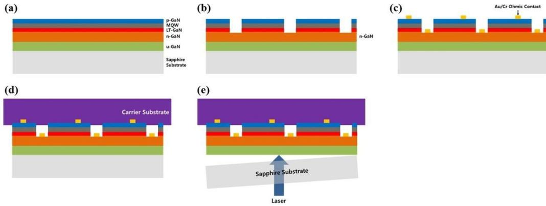
Figure 1. Schematic diagrams of laser lift-off for carrier substrate investigation
