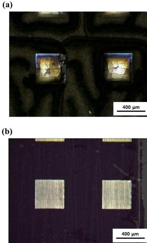
Figure 4. Laser lift offed surface of GaN LED arrays with different XeCl laser beam dimensions (a) 1.2mm x 1.2mm square laser beam (b) 3μm x 5cm line shape laser beam
