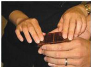
Braille screen fabricated on a plastic sheet.
