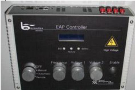
This stand-alone portable laboratory instrument simplifies the generation and control of high voltages for artificial muscle research. Features include 4 independent output channels, computer control, battery operation, and safety features that make it suitable for bench-top use.
