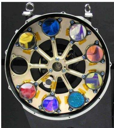
**Fig. 1.** Example of a set of optical interference filters fixed on a filter wheel and dedicated to the GOCI instrument installed on the COMS satellite [1]
