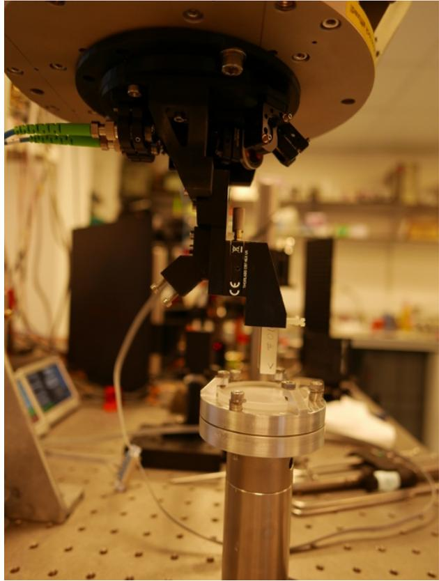
Figure 5. (Top Left) CAD assembly of the optical component holder and vertical interferometer mounted on a hexapod. All dimensions are in mm. (Bottom Left) Optical sketch, BSx are beamsplitters, BPF are bandpass filters, and QPD is a quadrant photodiode. (Right) A 3D printed assembly of a similar design mounted below a hexapod. The hexapod used here is for testing purposes, the final implementation will use a hexapod with a smaller footprint.
