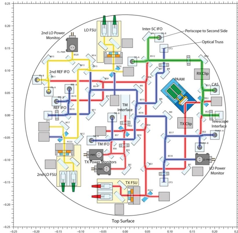
Figure 3. LISA Optical Bench concept (A-side). A representative preliminary design of the LISA optical bench. The design will evolve, but this gives a good idea of the complexity of the optical system which the facility is designed to build. The LISA optical bench is two sided; the side shown is the more complicated. Axis scales are in metres.
