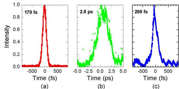
**Fig. 4** Pulse broadening in a DCPCF and the compression of the pulse width with dispersion precompensation. (a) Pulse from the laser; (b) pulse broadened after propagating in fiber; and (c) pulse compressed back with dispersion precompensation.
