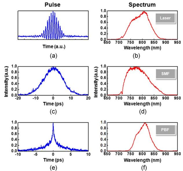
**Fig. 3** The pulse width and spectra of the laser beam measured before and after propagating through optical fibers. (a) and (b) Directly from the laser. (c) and (d) After propagating through 1.3-m SMF. (e) and (f) After propagating through 1.3-m hollow-core PBF.
