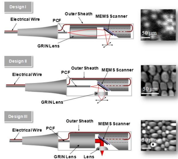
**Fig. 5** Three optical designs of the MPM probe and the corresponding images acquired with the designs. Design I: A GRIN lens is located before the MEMS mirror. Design II: A GRIN lens is located after the MEMS mirror. Design III: A GRIN lens and an aspheric lens are located before and after the MEMS mirror, respectively. All images show  $20\text{-}\mu\text{m}$  fluorescent microspheres. The scale bar is  $50 \mu\text{m}$ .
