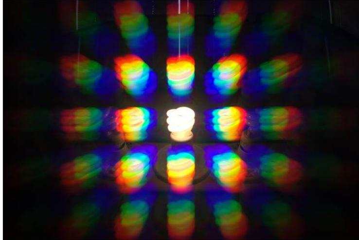
Figure 8. A 3500K compact fluorescent lamp as viewed through a transmissive diffraction grating.
