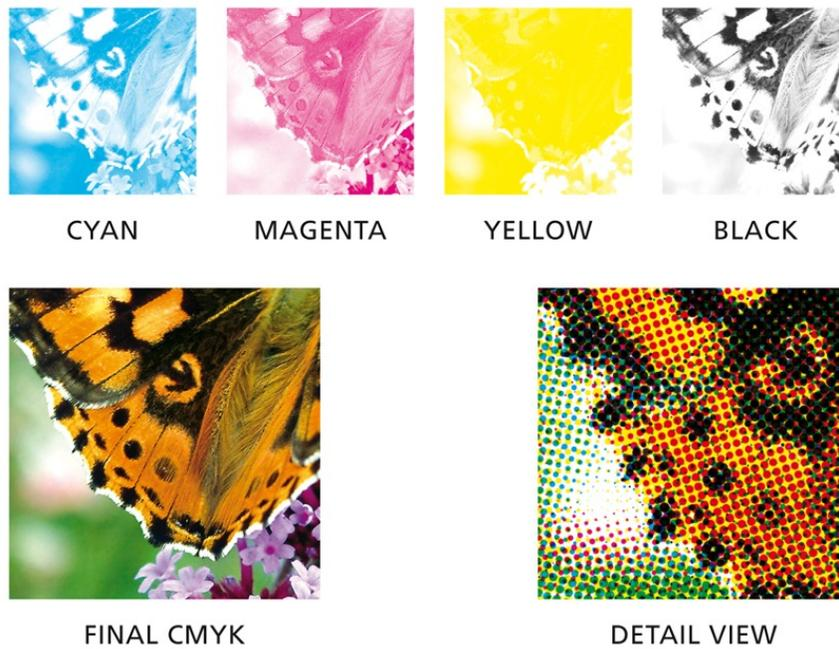
Figure 13. The typical CMYK printing process and the resulting dot patterns. [15]
