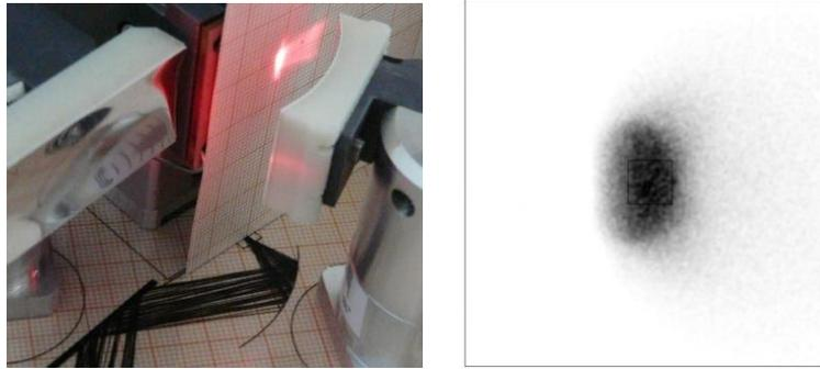
Figure 11. Comparison of the imaged beam spot at the target with the simulated irradiance distribution.
