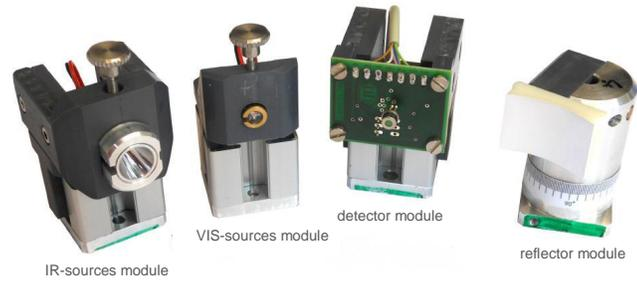
Figure 8. Modules of the IR-gas sensor construction kit.
