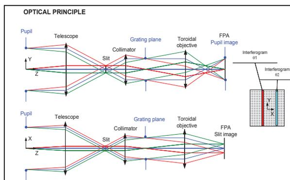
Fig.1 Optical concepts of heterodyne imaging spectrometer
