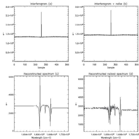
Fig.3 Initial spectrum ( c ) and its interferogram ( a ).
