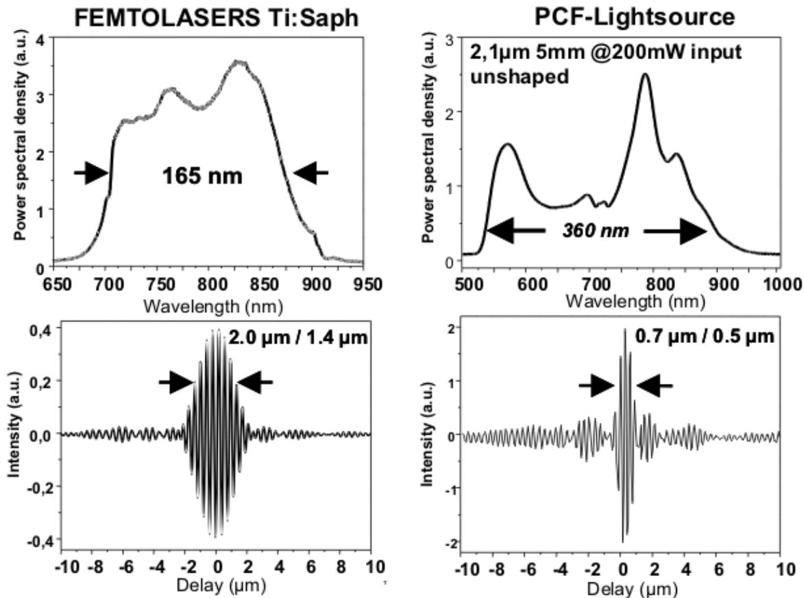
**Figure 2** Optical spectra (top) and interference signals (bottom) of a commercially available Ti:sapphire laser (Femtsource Compact Pro, FEMTOLASERS; left) and a photonic crystal fiber based light source (right). An axial resolution of 2.0  $\mu\text{m}$  and 0.9  $\mu\text{m}$  in free space, corresponding to about 1.4  $\mu\text{m}$  and 0.6  $\mu\text{m}$  in biological tissues can be achieved with the Ti:sapphire and the photonic crystal fiber optically based light source, respectively.
