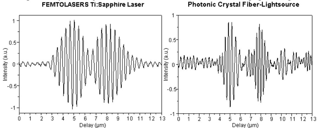
**Figure 3 .** Measurement of nitrocellulose membrane thickness with a Ti:sapphire laser (Femtosource Compact PRO, FEMTOLASERS; left) and a photonic crystal fiber based light source (right) demonstrating the potential for ultrahigh resolution OCT imaging. An optical thickness of 3.3  $\mu\text{m}$ , i.e. a geometrical thickness of 2.2  $\mu\text{m}$  ( $n_g \sim 1.5$ ) has been achieved.
