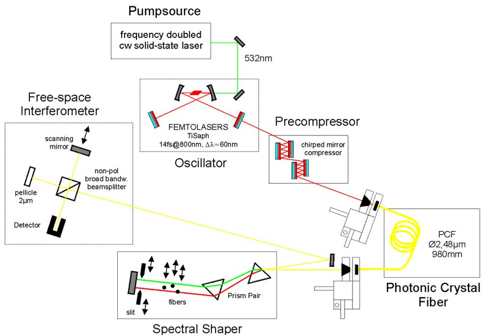
**Figure 1** Schematics of the photonic crystal fiber light source based OCT setup. The oscillator and fiber parameters are optimized for visible light emission. An external prism sequence is used to spectrally shape the pulses. A free space interferometer is designed for ultrabroad bandwidths in the visible wavelength range to achieve sub-micrometer axial resolution.
