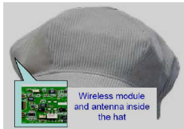
**Figure 11. Wireless module and antenna on hat.**
