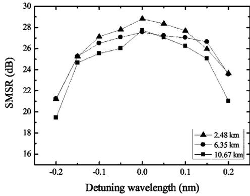
**Fig. 2** SMSR with several lengths between the ONU and the RN. SMSR at each bias setting:  $1.28 I_{th}$  ( $\blacktriangle$ ),  $1.29 I_{th}$  ( $\bullet$ ), and  $1.33 I_{th}$  ( $\blacksquare$ ).
