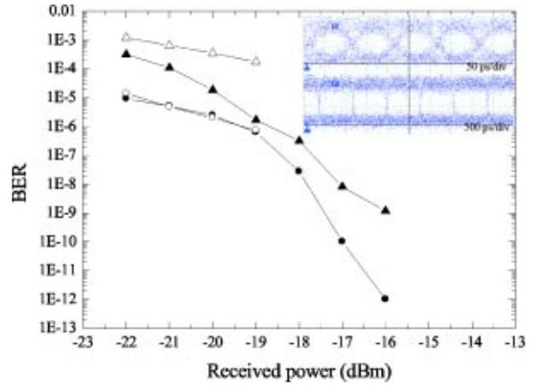
**Fig. 4** Measured BER curves for the upstream signal at 1.25/10 Gbit/s with PRBS of  $2^7 - 1$ . Self-locked F-P LD: at 1.25-Gbit/s ( $\bullet$ ), at 10-Gbit/s ( $\blacktriangle$ ). F-P LD: at 1.25-Gbit/s ( $\circ$ ), at 10-Gbit/s ( $\triangle$ ). Inset: self-locked eye diagrams at 1.25 (lower: 500 ps/div), 10 Gbit/s (upper: 50 ps/div).
