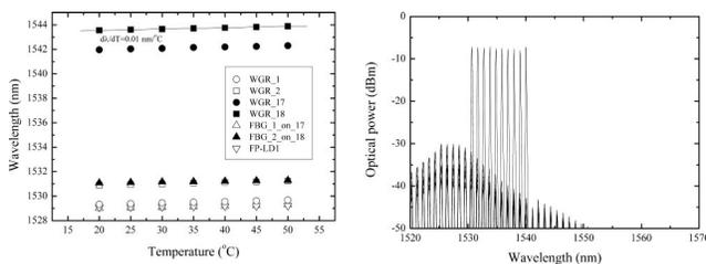
**Fig. 3** Dependence of wavelength on temperature and tuning range of the F-P LD. (a) WGR ( $\circ$ ,  $\square$ ,  $\bullet$ ,  $\blacksquare$ ), FBG ( $\triangle$ ,  $\blacktriangle$ ), and the self-tuned F-P LD ( $\nabla$ ). (b) Tuning range of single F-P LD for multiple ONUs.
